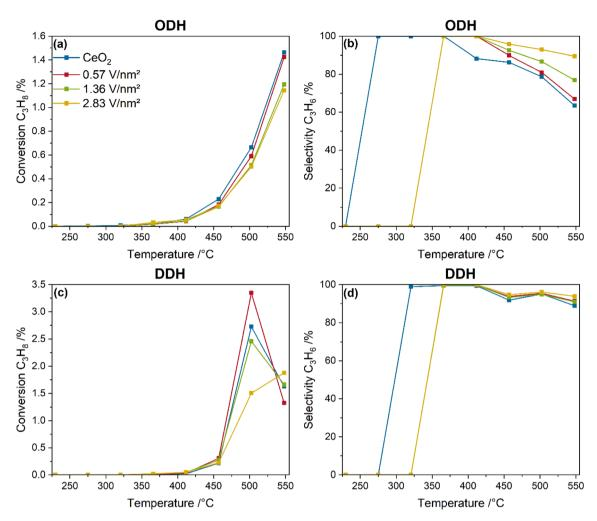
Fig. 1 Comparison between the temperature-dependent conversions (a and c) and selectivities (b and d) of bare ceria and vanadia-loaded samples between 225 and 550 °C under ODH (12.5%  $CO_2/12.5\%$   $C_3H_8/He$ ) and DDH (12.5%  $C_3H_8/He$ ) conditions.
