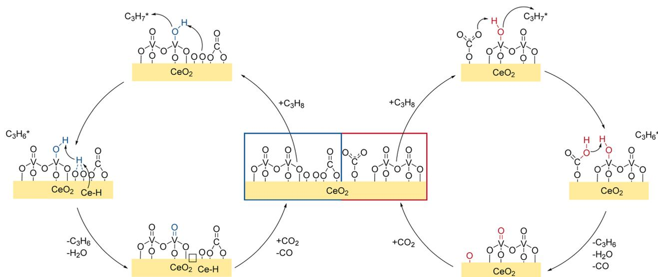
Fig. 9 Mechanistic scheme of the CO<sub>2</sub>-assisted propane ODH over VO<sub>x</sub>/CeO<sub>2</sub>. Details regarding the role of the bare support and side reactions are given in the text.
