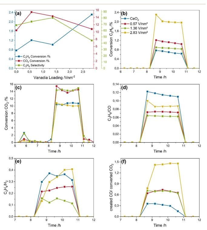
Fig. 3 Analysis of the CO<sub>2</sub>-assisted propane ODH reaction network over bare ceria and vanadia-loaded samples: (a) loading-dependent propane and  $CO_2$  conversions and propylene selectivities, (b) propane and (c)  $CO_2$  conversions, and (d) propylene/CO, (e) ethylene/ $H_2$  and (f) created CO/converted CO2 ratios.
