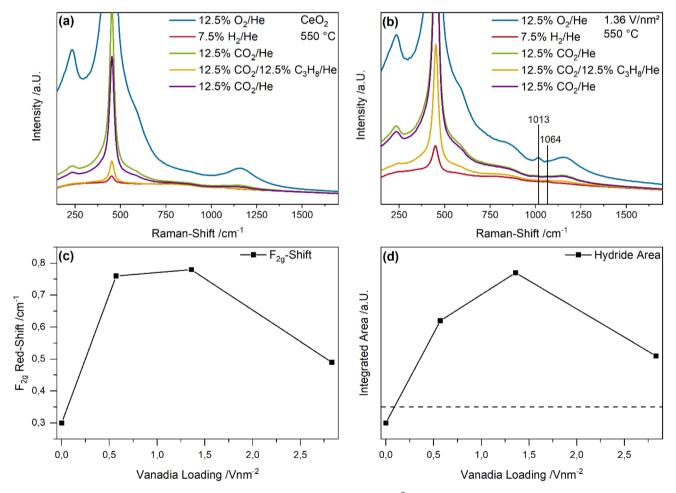
Fig. 5 Vis-Raman spectra (514 nm excitation) of (a) bare ceria and (b) the 1.36 V nm<sup>-2</sup> samples under different gas feeds recorded at 550 °C. (c) The F<sub>2q</sub> shift and (d) the hydride areas were determined by fitting and integration. The dashed line in panel d indicates no intensity change. For details see text
