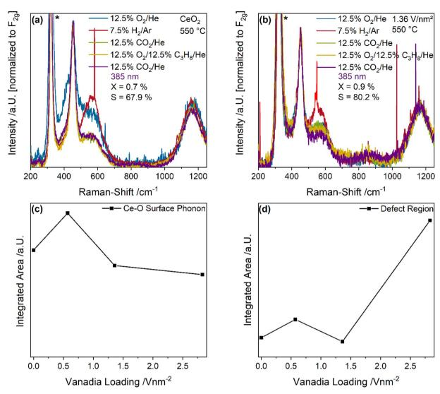
Fig. 4 UV-Raman spectra (385 nm excitation) of (a)  $CeO_2$  and (b) the 1.36 V nm<sup>-2</sup> sample recorded under the indicated gas feeds at 550 °C. Spectra were normalized to the  $F_{2g}$  peak and the  $CaF_2$  window signal is marked with an asterisk. Quantification of the (c) Ce-O surface phonon and (d) defect region changes between spectra recorded under 12.5%  $CO_2/He$  and 12.5%  $CO_2/12.5\%$   $C_3/He$ 8.
