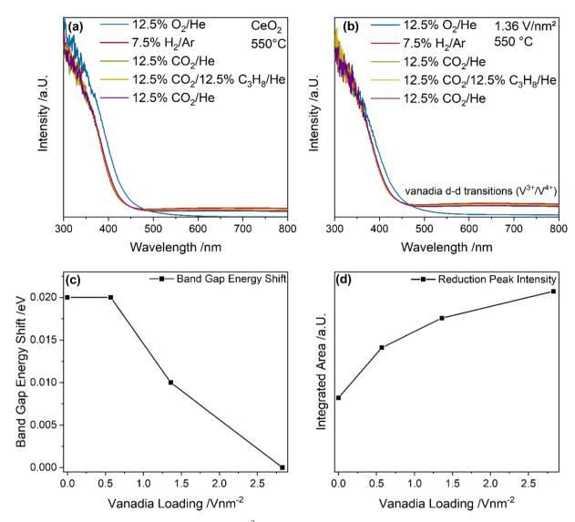
Fig. 7 UV-Vis spectra of (a) bare ceria and (b) the 1.36 V nm<sup>-2</sup> sample under different gas feeds, recorded at 550 °C. (c) Band gap energies as determined using Tauc plots and (d) the reduction peak area based on the results of a fitting analysis.
