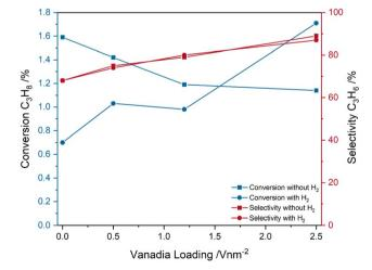
Fig. 2 Comparison between the conversions and selectivities of bare ceria and vanadia-loaded samples after different pre-treatments (fully oxidized with  $O_2$  and partially reduced with  $H_2$  and subsequently regenerated with  $H_2$  conditions (12.5%  $H_2$ ) under ODH conditions (12.5%  $H_2$ ) at 550 °C.
