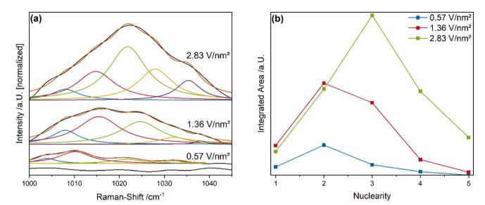
Fig. 6 (a) Vanadyl region from the Vis-Raman spectra (514 nm excitation) between 1000 and 1045 cm $^{-1}$  for bare ceria and vanadia-loaded samples during 12.5%  $O_2$ /He exposure at 550 °C together with the results of peak-fit analyses. (b) Loading-dependent nuclearity distribution based on the analyses shown in (a). For details see text.
