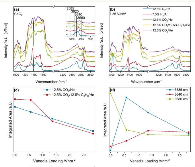
Fig. 8 Quasi in situ DRIFT spectra of (a)  $CeO_2$  and (b) the 1.36 V nm $^{-2}$  sample recorded after treatment under the indicated gas feeds at 550 °C and subsequent cooling to room temperature in helium. The inset shows an enlarged view of the Ce-OH region. (c) Carbonate areas during the first  $CO_2$ /He and the reactive gas phase and (d) relevant Ce-OH peaks, which show a significant change in intensity upon switching from 12.5%  $CO_2$ /He to 12.5%  $CO_2$ /12.5%  $CO_2$ /12.5%
