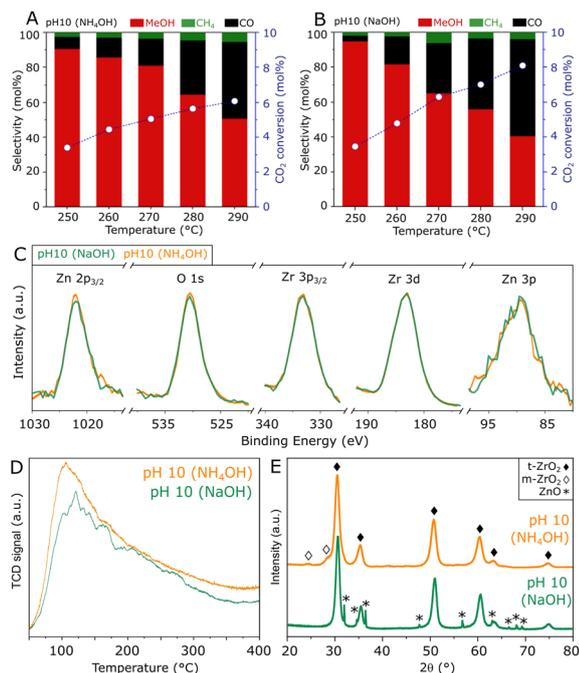
Fig. 5 Comparison of  $\text{ZnZrO}_x$  catalysts produced under synthesis pH 10 with the distinct additives  $\text{NH}_4\text{OH}$  and  $\text{NaOH}$ , in terms of  $\text{CO}_2$  hydrogenation performance (A and B),  $\text{Zn } 2p_{3/2}$ ,  $\text{O } 1s$ ,  $\text{Zr } 3p_{3/2}$ ,  $\text{Zr } 3d$  and  $\text{Zn } 3p$  XPS spectra (C),  $\text{CO}_2$ -TPD profiles (D) and XRD patterns (E).
