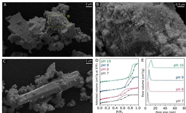
Fig. 2 SEM micrographs of ZnZrO<sub>x</sub> produced at pH10 under different magnifications (A and B) and the region including rod-like particles (C). N<sub>2</sub> sorption isotherms (D) with respective pore size distributions of ZnZrO<sub>x</sub> produced at pH 7, 8, 9 and 10 (E).
