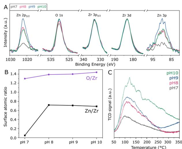
Fig. 3 Survey XPS spectra of ZnZrO<sub>x</sub> normalized by the Zr 3d peak, showing the Zn 2p<sub>3/2</sub>, O 1s, Zr 3p<sub>3/2</sub>, Zr 3d and Zn 3p regions (A) with the respective quantification of the Zn/Zr and O/Zr surface molar ratios (B); CO<sub>2</sub>-TPD profiles of the samples produced at pH 7 to 10 (C).
