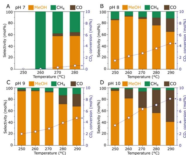
Fig. 4 CO<sub>2</sub> hydrogenation performance of ZnZrO<sub>x</sub> catalysts produced under synthesis pH 7 (A), 8 (B), 9 (C), and 10 (D). Reaction conditions: 0.5 g catalyst, 2.0 MPa, CO<sub>2</sub>/H<sub>2</sub> = 1/3, 5 mL min<sup>-1</sup>.
