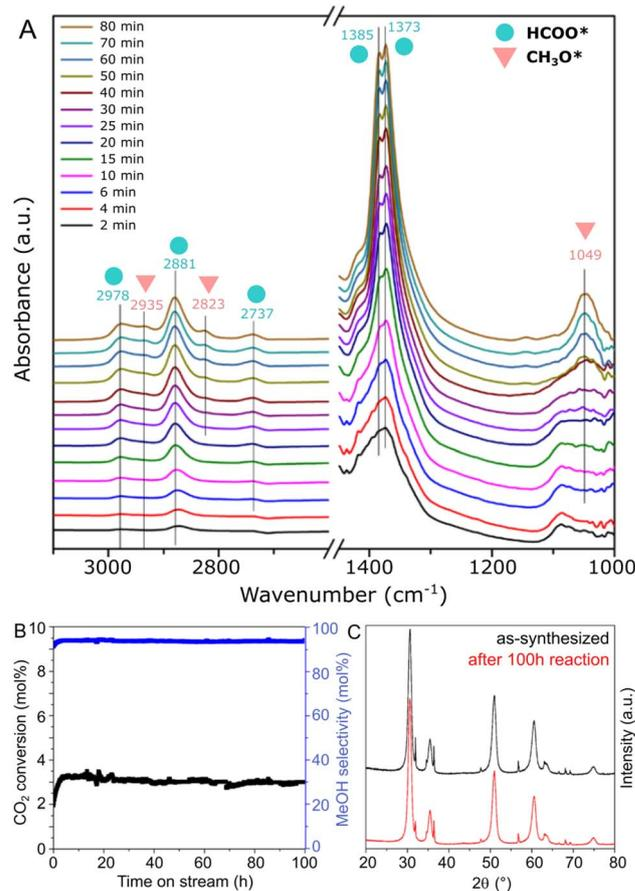
Fig. 6 *In situ* DRIFTS results of  $\text{CO}_2$  hydrogenation conditions at 250 °C (A) and catalytic stability test at 250 °C using the  $\text{ZnZrO}_x$  catalyst produced at pH 10 with  $\text{NaOH}$  (B), with the respective XRD patterns of as synthesized and spent material (C).
