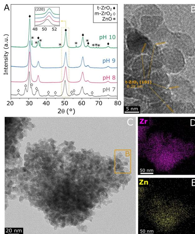
Fig. 1 XRD patterns of ZnZrO<sub>x</sub> produced at different synthesis pH values and calcined at 500 °C (A), TEM image of ZnZrO<sub>x</sub> produced at pH 8 (B and C) and TEM-EDX mapping images showing the Zr and Zn distribution in the same region covered by C (D and E).
