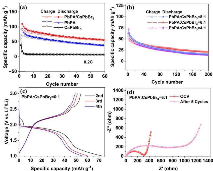
Fig. 2 Electrochemical characterization. (a) Cycling performance of the batteries based on PbPA, CsPbBr<sub>3</sub>, and PbPA : CsPbBr<sub>3</sub> = 6 : 1 at 0.2C (1C = 100 mA h g<sup>-1</sup>). (b) Cycling performance of the batteries based on PbPA : CsPbBr<sub>3</sub> = 4 : 1, 6 : 1, and 8 : 1 at 0.2C. (c) Charge/discharge profiles of the PbPA : CsPbBr<sub>3</sub> = 6 : 1 battery. (d) EIS spectra of the pristine PbPA : CsPbBr<sub>3</sub> = 6 : 1 battery and that after working for five cycles.
