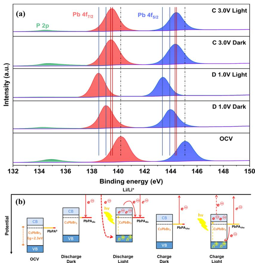
Fig. 5 Photo-assisted working mechanism. (a) XPS Pb 4f and P 2p spectra of the PbPA : CsPbBr<sub>3</sub> = 6 : 1 cathode under different conditions. (b) Energy alignment and the carrier flow in the system.
