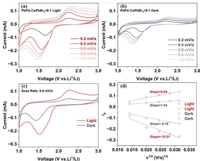
Fig. 4 Electrochemistry profiles of the quasi-solid-state PA-LIB based on PbPA : CsPbBr<sub>3</sub> = 6 : 1 working under different conditions. CV curves at different scan rates (0.2–1.0 mV s<sup>-1</sup>) measured under light illumination (a) and in the dark (b). (c) CV curves at a scan rate of 0.6 mV s<sup>-1</sup> with and without light. (d) Diffusion constant analysis under dark and light conditions.
