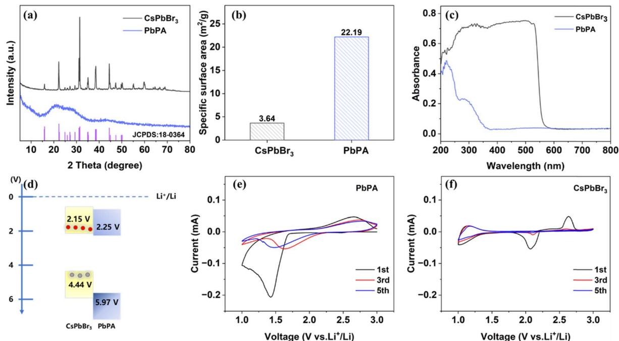
Fig. 1 Physical characterization. (a) XRD patterns. (b) Specific surface area. (c) UV-vis absorption spectra of PbPA and CsPbBr<sub>3</sub>. (d) Band diagram of the two units. (e and f) CV curves at 0.2 mV s<sup>-1</sup> for the first, third and fifth cycle of PbPA and CsPbBr<sub>3</sub>.
