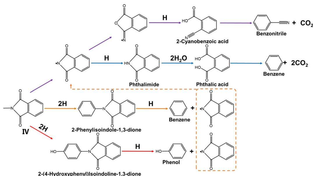
Fig. 6 The pyrolysis reaction pathway of intermediate IV.
