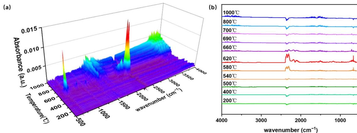
Fig. 3 (a) 3D FT-IR and (b) 2D FT-IR mapping data of the TG exit gas at a  $10 \text{ K min}^{-1}$  heating rate at the onset of pyrolysis.
