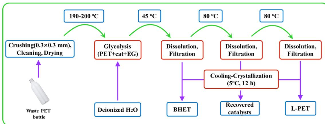
Fig. 2 The operation steps of the experiment.
