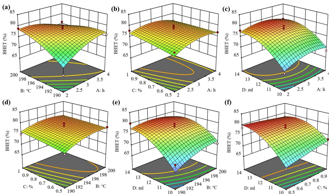
Fig. 7 Diagram of RSM between the various factors. (a): time and temperature; (b): time and catalyst dosage; (c): time and EG volume; (d): temperature and catalyst dosage; (e): temperature and EG volume; (f): catalyst dosage and EG volume.
