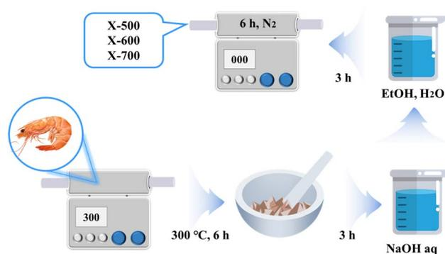
Fig. 1 Preparation of the shrimp shell derivative catalyst.
