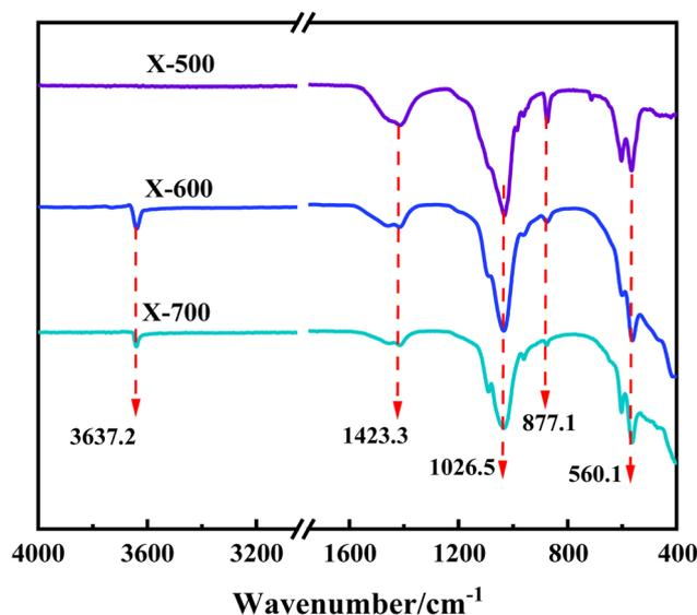
Fig. 3 FT-IR spectra of X-500, 600, and 700.
