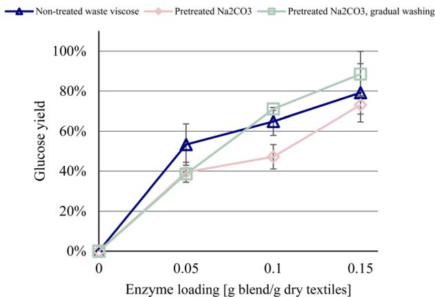
Fig. 4 Glucose yield of alkali pretreated post-consumer waste viscose (70 °C, 1 h, 5% Na<sub>2</sub>CO<sub>3</sub>) with and without gradual washing.
