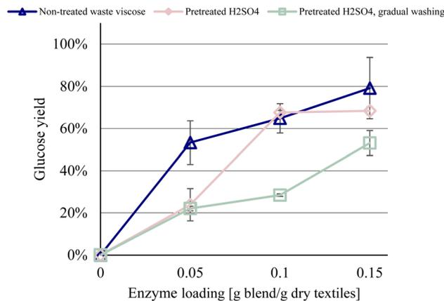
Fig. 5 Glucose yield of acid pretreated post-consumer waste viscose (30 °C, 30 min, 15% H<sub>2</sub>SO<sub>4</sub>) with and without gradual washing.
