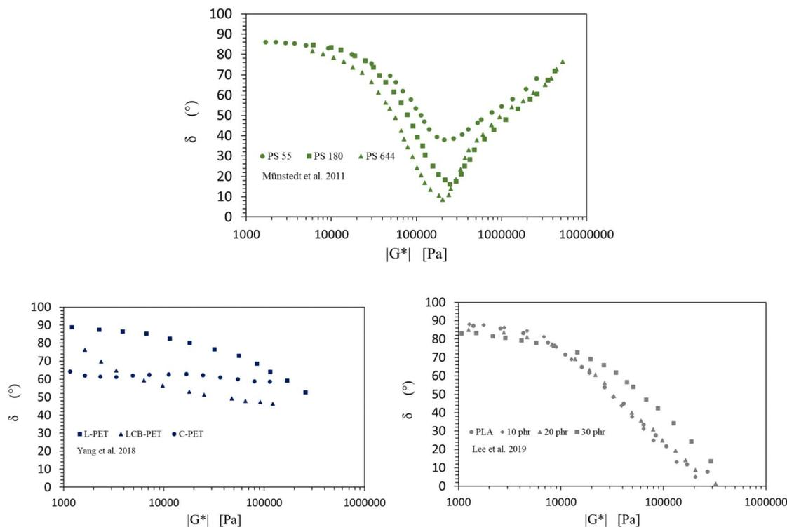
Fig. 32 Van Gorp-Palmen (vGP) plots (phase angle  $\delta$  as a function of complex modulus  $|G^*|$ ) for (top) three polystyrene (PS) samples with different average molar masses; for (bottom left) linear PET (L-PET), branched PET (LCB-PET) and cross-linked PET (C-PET); and for (bottom right) neat PLA and PLA modified with acrylic core-shell rubber (filler content in phr). Data to construct the subfigures taken from ref. 192–194.
