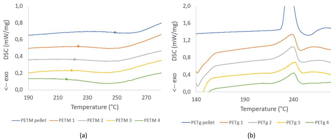
Fig. 44 DSC curves for TGA analysis of PETM (a) and PETg (b) sample residence time with the oxidation onset temperature highlighted based on Trossaert *et al.*<sup>217</sup> Both subplots are reproduced in open access redistribution mode.
