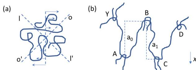
Fig. 11 Conceptual illustration of why melts are prone to thermo-mechanical degradation, with an isolated polymer chain under shear flow (a) having flexibility and a chain having entanglements in the melt ((b); concentrated cases), experiencing stress points for shear-induced breakage.<sup>114</sup>
