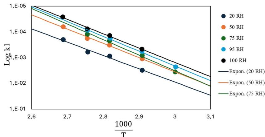
Fig. 23 Arrhenius parameter plots for PET hydrolysis at different relative humidity (RH) percentages.<sup>155</sup> The figure is constructed based on the data by McMahon *et al.*<sup>155</sup>
