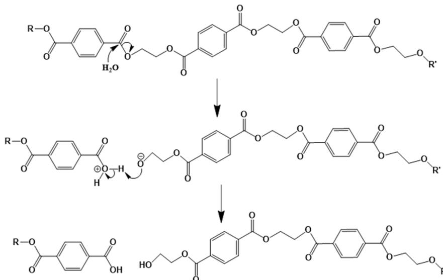
Fig. 19 Mechanism of PET hydrolytic degradation based on the work by Sammon *et al.*<sup>139</sup>
