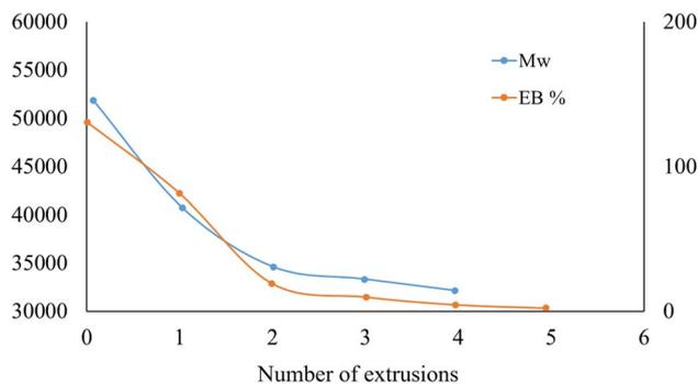
Fig. 45 Mass average molar mass (or molecular weight;  $M_w$ ) and elongation (EB) at break after different extrusion cycles for PET. Data to construct the figure were taken from La Mantia *et al.*<sup>108</sup>
