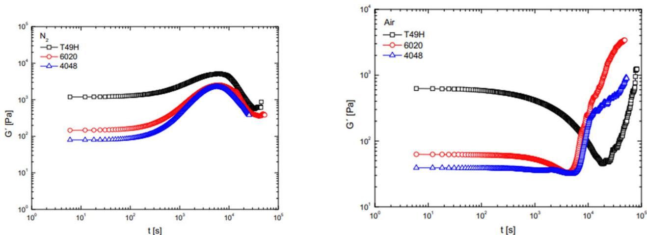
Fig. 31 Storage modulus ( $G'$ ) measured as a function of time in the presence of nitrogen (left) and air (right) of 3 different PET grades: PET T49H (black), 6020 (red) and 4048 (blue). Temperature of 280 °C, frequency of 10  $\text{rad s}^{-1}$  and deformation of 10%.<sup>188</sup> Reproduced with permission from the publisher, AIP Publishing.
