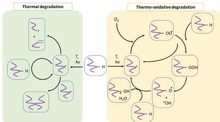
Fig. 5 Typical reactions for thermal degradation (left) and thermo-oxidative degradation (right), starting from a general polymer “purple” chain depicted in the middle;  $T$ : temperature;  $h$ : the Planck constant and  $\nu$ : frequency.
