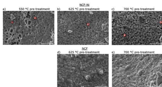
**Fig. 5** SEM images of NCF (d and e) and NCF-Ni (a–c) after a reductive pre-treatment at 550 °C (a), 625 °C (b and d), and 700 °C (c and e) followed by DRM up to 950 °C, respectively. While for NCF-Ni, some nanoparticles are still visible after the reaction (red circles), the oxide backbone of the catalyst underwent dramatic changes compared to the images after the reduction (Fig. 2).
