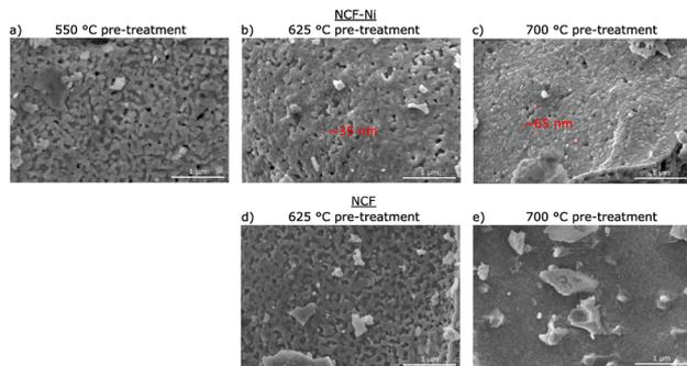
Fig. 2 SEM images of NCF (d and e) and NCF-Ni (a–c) after a reductive pre-treatment at 550 °C (a), 625 °C (b and d) and 700 °C (c and e) respectively. For NCF-Ni, the size of the exsolved nanoparticles (red circles) increases with the rising temperature of the pre-treatment. For NCF, no exsolution is visible even after 700 °C pre-treatment.
