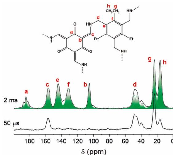
**Fig. 1** <sup>1</sup>H–<sup>13</sup>C CP MAS NMR spectra of POP-W-Et performed at variable contact time and a spinning speed of 12.5 kHz.
