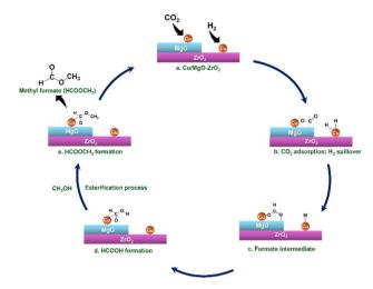
**Scheme 2** Plausible mechanism for the hydrogenation of CO<sub>2</sub> to MF in the presence of MeOH over the Cu/MqO–ZrO<sub>2</sub> catalyst.
