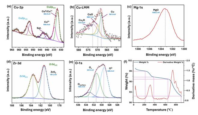
XPS patterns for (a) Cu 2p, (b) Cu LMM, (c) Mg 1s (d) Zr 3d, and (e) O 1s; (f) TGA profile of 5C-20MZ
