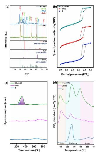
Fig. 3 (a) XRD diffractograms of 20MZ and 5C-20MZ, (b) N<sub>2</sub> physisorption isotherms of Z. 20MZ, 5C-20MZ, (c) H<sub>2</sub>-TPR profiles of Z. 20MZ, and 5C-20MZ, and (d) CO<sub>2</sub>-TPD profiles of Z, 20MZ, and 5C-20MZ.
