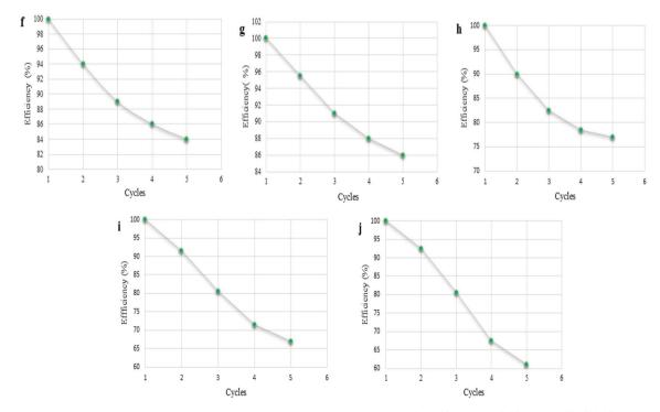
Fig. 2 Variation of the catalytic efficiency as function of the catalyst reuse times (cycles) for (f) DABCO, (g) [H-dabco][Cl], (h) [H-dabco][AcO], (i) DABCO-CuCl, and (j) DABCO-CuI in the model reaction between EAA 1 and salicylaldehyde 2a in the presence of water.
