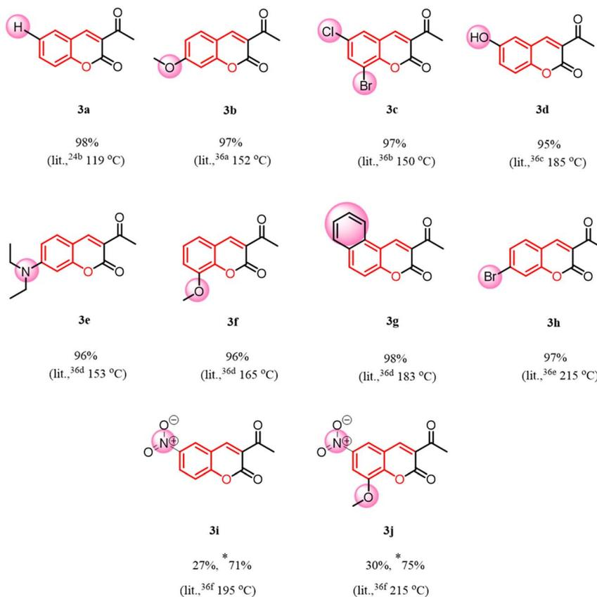
**Scheme 2** Scope of the reaction of *o*-hydroxyaldehydes **2a–h** with EAA **1** employing different catalysts. % Yield taken in the gram scale and melting point in °C. \*Heating (65–70 °C), \*\*literature value.<sup>24b,36a–f</sup>
