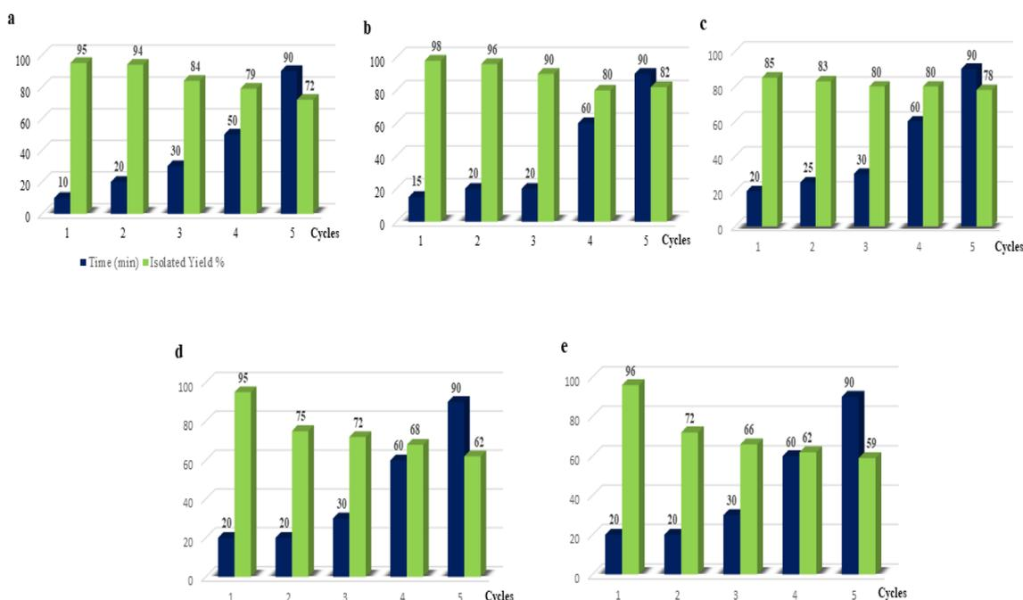
**Fig. 1** Reuse of the catalysts (a) DABCO, (b) [H-dabco][Cl], (c) [H-dabco][AcO], (d) DABCO–CuCl, and (e) DABCO–CuI in the model reaction between EAA 1 and salicylaldehyde 2a in the presence of water.
