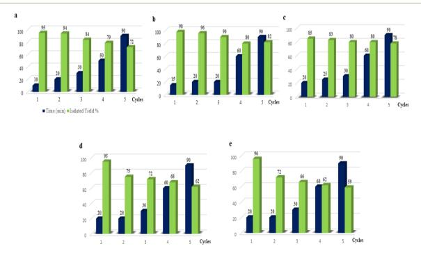
Fig. 1 Reuse of the catalysts (a) DABCO, (b) [H-dabco][CI], (c) [H-dabco][AcO], (d) DABCO-CuCl, and (e) DABCO-Cul in the model reaction between EAA 1 and salicylaldehyde 2a in the presence of water.
