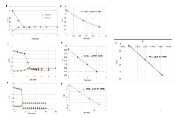
Fig. 6 (T–V) Reaction profiles for the experiments conducted and listed as entries 1–3 in Table 6. (W–Y) Regression plots of OD vs. time. (Z) Plot of  $\log[k]$  vs. [1\7] in determining the activation parameters. The solid red dots indicate the reactant and the green dots are for the product.
