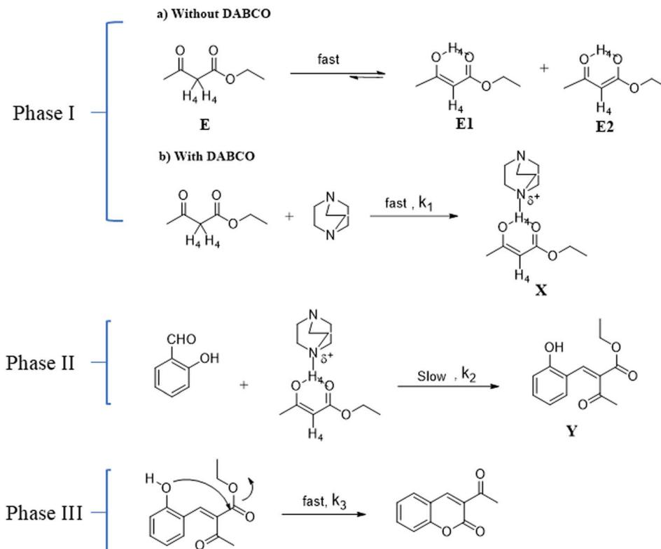
Fig. 7 Proposed reaction mechanism.
