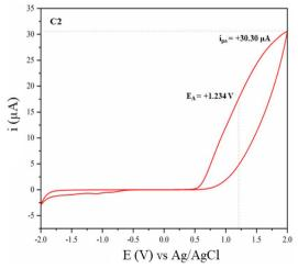
Fig. 10 Plot of the current vs. potential: C1 represents the quasi-reversible tautomerism of EAA, C2 represents the arrested form of EAA-DABCO a favoured irreversible reaction.
