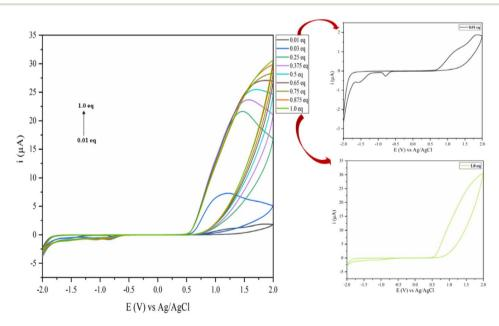
Fig. 12 Plot of the current vs. potential showing the conversation of the quasi-reversible to an irreversible process with increasing the concentration of DABCO (from 0.0125 to 1 eq.).
