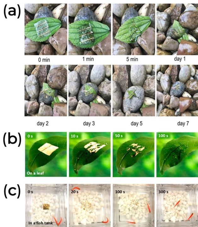
Fig. 10 (a) The degradation process of a chlorophyll-a/SWCNT composite transistor in a natural environment. Reprinted with permission from Q. Ou *et al.*<sup>150</sup> Copyright 2021, John Wiley and Sons. (b and c) The pectin-based synaptic transistor degradability. Reprinted with permission from Y. Li *et al.*<sup>159</sup> Copyright 2022, American Chemical Society.
