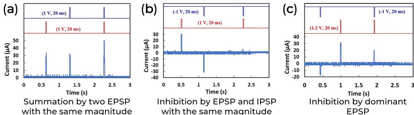
Fig. 9 Synaptic integration in a spatial summation configuration of an ITO/Honey/Ag 2-T neuromorphic device. Adapted with permission from B. Sueoka *et al.*<sup>78</sup> Copyright 2022, AIP publishing.
