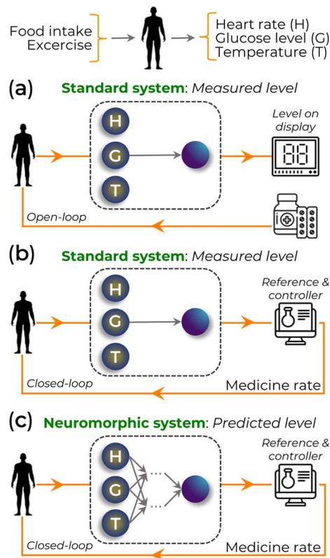
Fig. 15 Schematic of (a) open-loop and (b and c) closed-loop systems based on bioelectronics sensing, inspired by.<sup>196</sup> These systems (a and b) are related to the traditional method of measuring the glucose level without considering other parameters. In (c), the glucose level is estimated considering multiple and interconnected variables.
