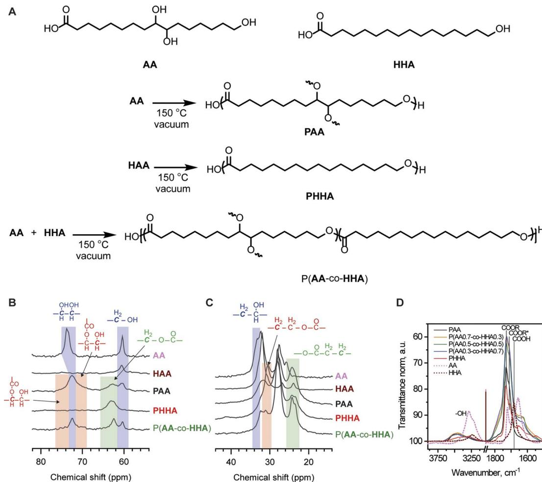
Fig. 1 (A) Chemical structures of monomers AA and HHA and polymers PAA, PHAA, and P(AA-co-HHA) obtained from melt polymerization or copolymerization. (B and C) Overlaid solid-state  $^{13}\text{C}$  NMR spectra of monomers and polyesters. (D) Overlaid FT-IR spectra of monomers and copolymers, where transmittance values were normalized to the antisymmetric vibration of methylene functional groups at  $2925\text{ cm}^{-1}$ .
