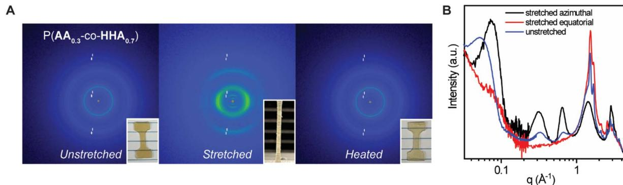
Fig. 4 (A) 2D WAXS images of P(AA<sub>0.3</sub>-co-HHA<sub>0.7</sub>) of unstretched, stretched, and, after the heating. (B) 1D SAXS/WAXS curves for P(AA<sub>0.3</sub>-co-HHA<sub>0.7</sub>) in the stretched and unstretched states where azimuthal and equatorial curves are reported for stretched sample.
