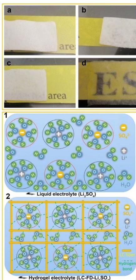
Fig. 3 Upper panel: optical image of an LC membrane (a), LC-FD membrane (b), LC membrane-based hydrogel electrolyte LC- $\text{Li}_2\text{SO}_4$  (c) and LC-FD membrane-based hydrogel electrolyte LC-FD- $\text{Li}_2\text{SO}_4$  (d). Lower panel: schematic diagram of the liquid electrolyte (1) and hydrogel electrolyte (2). Adapted from Qiu *et al.* (2020).<sup>42</sup> Copyright 2020, Elsevier Ltd.
