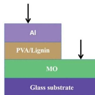
Fig. 8 Vertical sandwich structure of Mo/lignin and PVA film/Al. Adapted from W. Zhang *et al.* (2023).<sup>65</sup> Copyright 2023, IEE.
