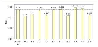
Fig. 14 CoF values of Group III+ base oil, and its formulations containing 1 wt% of GMO or saturated solutions of boronium ILs; data recorded between 1800 and 3600 s.
