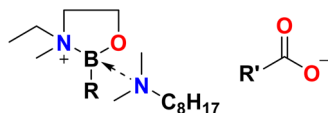
Fig. 1 The general formula of task-specific triboactive ionic liquids ( R, R' – alkyl chains).
