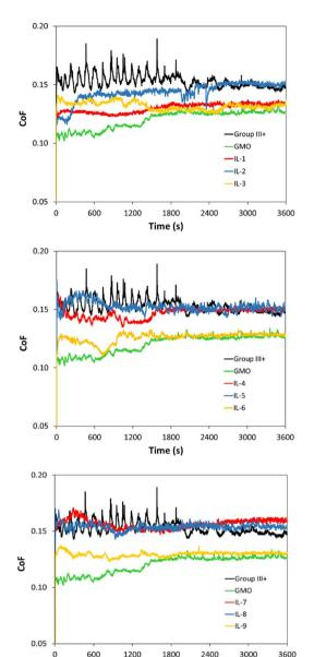
Fig. 13 CoF profiles of saturated solutions of boronium ILs in Group III+ base oil, compared to neat Group III+. Top:  $[B(C_{2mea})(n-Bu)]^+$  ILs, middle:  $[B(C_{2mea})(sec-Bu)]^+$  ILs and bottom:  $[B(C_{2mea})(sec-Bu)]^+$  ILs. Anions: 2-ethylhexanoate (IL-1, 4 and 7), methacrylate (IL-2, 5 and 8) and oleate (IL-3, 5 and 9).
