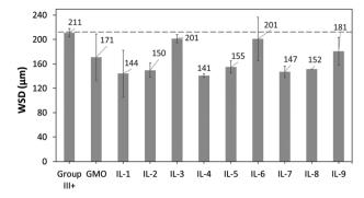
Fig. 16 WSD values of metal ball specimens obtained after HFRR tests, from neat Group III+ and its formulations with 1 wt% of GMO or saturated solutions of boronium II s
