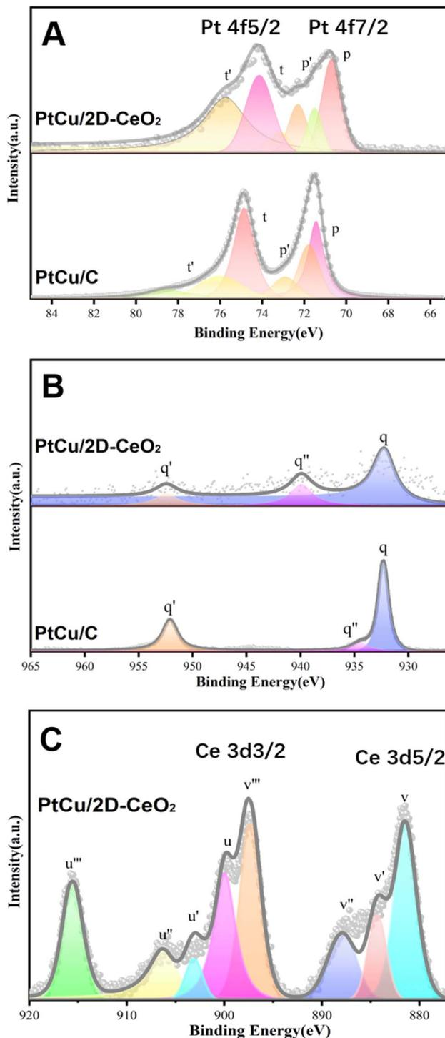
Fig. 3 XPS spectra of Pt 4f (A), Cu 2p (B), and Ce 3d of PtCu/2D-CeO<sub>2</sub> (C) orbitals.
