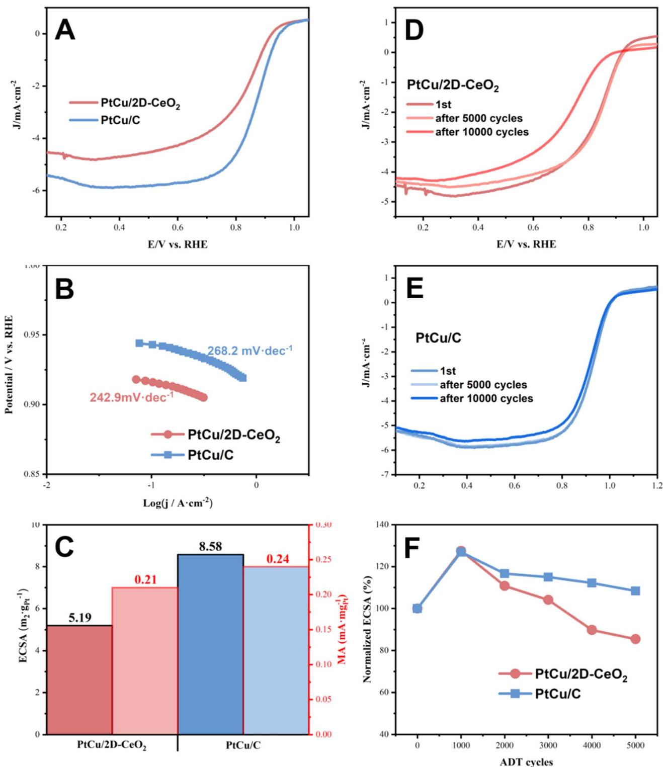
Fig. 5 The LSV curves (A), Tafel slopes (B), and ECSA and MA (C) of PtCu/C and PtCu/2D-CeO<sub>2</sub>; LSV curves of PtCu/2D-CeO<sub>2</sub> (D) and PtCu/C (E) 10 000 ADT cycles; and normalized ECSA (F).
