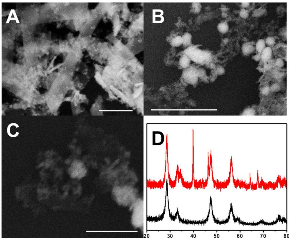
Fig. 1 (A) The SEM images of 2D-CeO<sub>2</sub>; (B) 2D-CeO<sub>2</sub> supported Cu; (C) 2D-CeO<sub>2</sub> supported PtCu, and (D) the XRD of PtCu/2D-CeO<sub>2</sub> (red line) and CeO<sub>2</sub> (black line). The scale bars are 100 nm.
