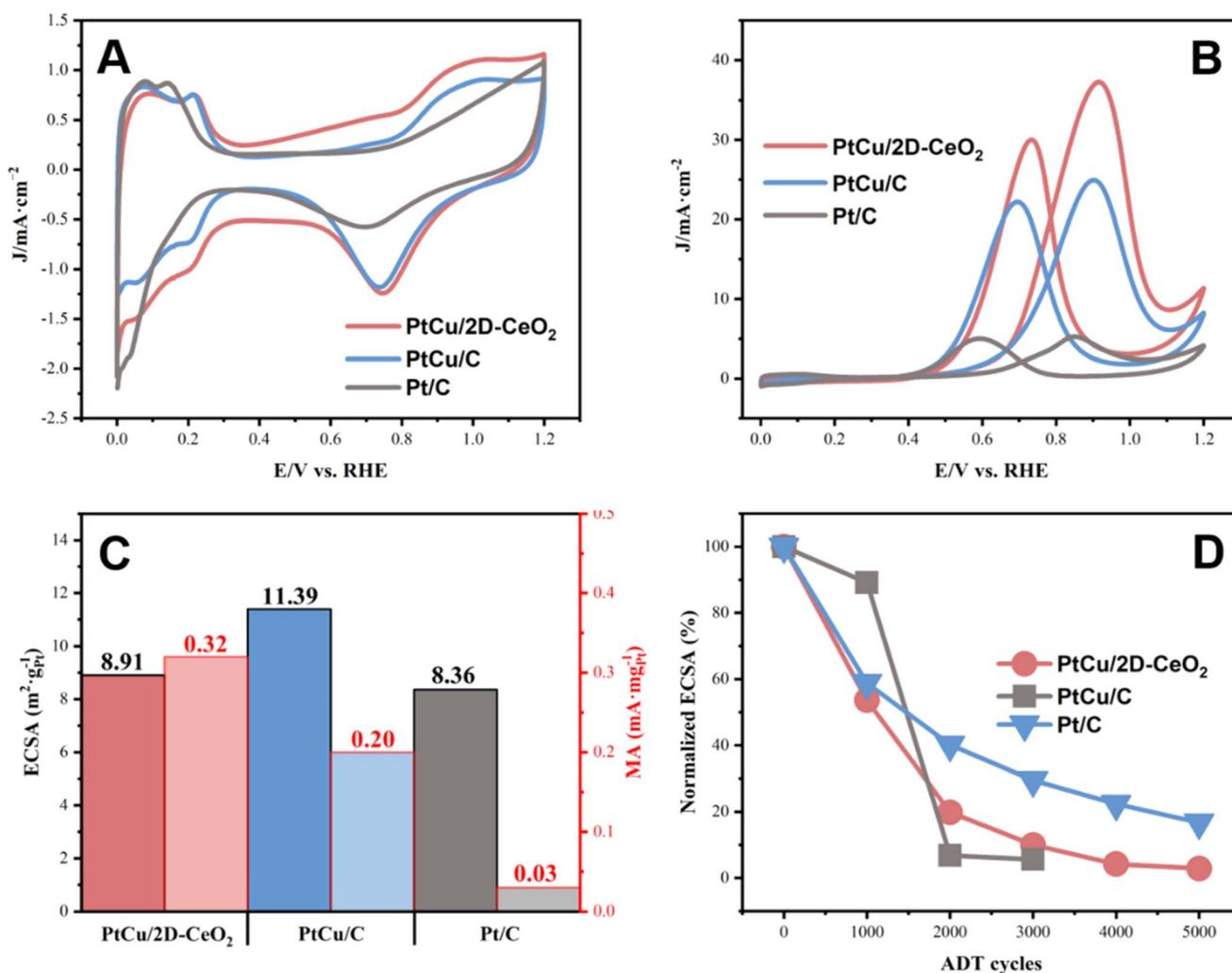
Fig. 4 The CV (A) and MOR (B) plots of PtCu/2D-CeO<sub>2</sub>, PtCu/C, and Pt/C; ECSA and MA diagrams of PtCu/2D-CeO<sub>2</sub>, PtCu/C, and Pt/C (C); the normalized ECSA after ADT cycling (D).
