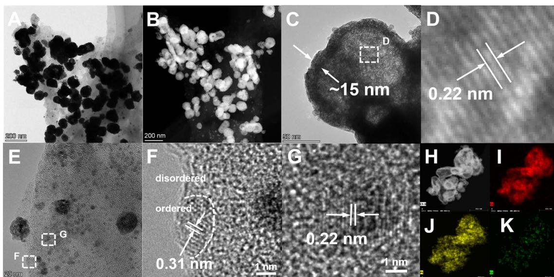
Fig. 2 TEM images of PtCu/2D-CeO<sub>2</sub> (A–G), and high-resolution images (C–G), the EDX element distribution (H–K).
