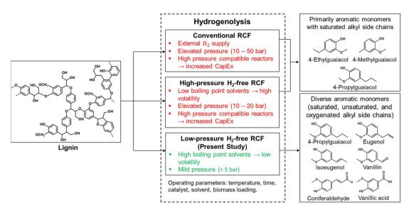
Scheme 1 Illustration of how this study (low pressure H<sub>2</sub>-free RCF) offers significant advancements in process safety, sustainability, and product range when compared to traditional RCF and high pressure H<sub>2</sub>-free RCF.
