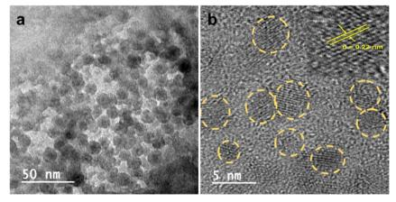
Fig. 2 (a) TEM image of Zn-Cdots (50 nm scale bar). (b) HRTEM image showing Zn-Cdots with an average size  $4.8 \pm 0.8$  nm (5 nm scale bar).
