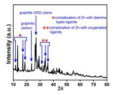
Fig. 3 The PXRD spectrum of Zn-Cdots.
