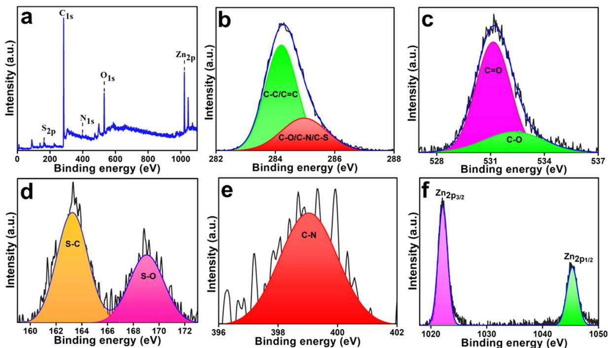
Fig. 4 (a) XPS full scan spectrum of Zn-Cdots. Deconvoluted high-resolution (b)  $\text{C}_{1\text{s}}$  signal (c)  $\text{O}_{1\text{s}}$  signal (d)  $\text{S}_{2\text{p}}$  signal (e)  $\text{N}_{1\text{s}}$  signal (f)  $\text{Zn}_{2\text{p}}$  signal.
