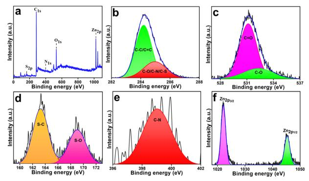
Fig. 4 (a) XPS full scan spectrum of Zn-Cdots. Deconvoluted high-resolution (b)  $C_{1s}$  signal (c)  $O_{1s}$  signal (d)  $S_{2p}$  signal (e)  $N_{1s}$  signal (f)  $Z_{1p}$  signal.
