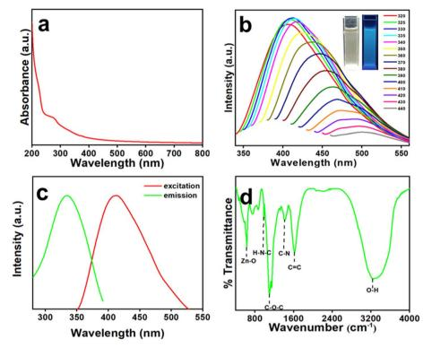
Fig. 1 (a) UV-Vis spectrum of Zn-Cdots dispersed in water at a concentration of 0.25 mg mL $^{-1}$ . (b) Excitation-dependent emission of Zn-Cdots dispersed in water at 0.5 mg mL $^{-1}$  concentration (inset: images of aqueous solution of Zn-Cdots under daylight and UV light). (c) Excitation (wavelength 330 nm) spectrum of Zn-Cdots corresponding to the 411 nm emission peak. (d) FTIR spectrum of Zn-Cdots.
