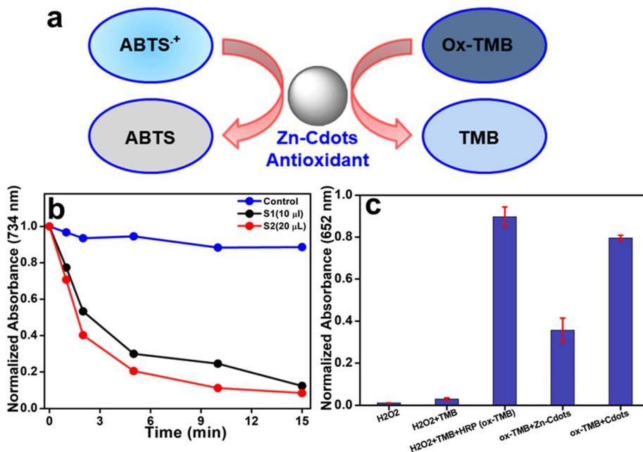
Fig. 7 (a) Schematic representation of antioxidant property of Zn-Cdots. (b) Time-dependent absorbance of ABTS radical (ABTS<sup>+</sup>) scavenging by Zn-Cdots at 734 nm. (c) Evaluation of antioxidant property of Zn-Cdots using TMB assay. The absorbance of Ox-TMB was measured at 652 nm.
