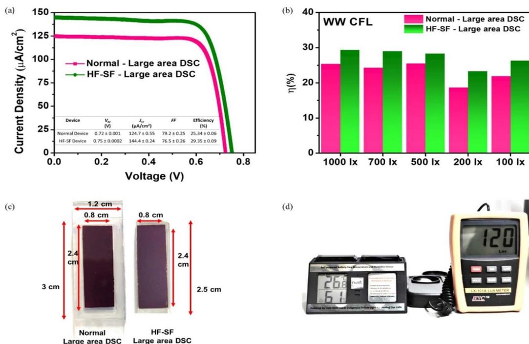
Fig. 3 (a)  $J$ - $V$  graph for large area DSCs under 1000 lux WW CFL illumination ( $J$ - $V$  data in the inset), (b) device performance of large area DSCs under WW CFL illumination (1000 lux–100 lux), (c) a comparison of normal large area DSCs with HF-SF large area DSCs and (d) a DSM made by serially interconnecting two large area DSCs powering an indoor weather monitoring unit (temperature and humidity sensor) under 120 lux indoor LED illumination.
