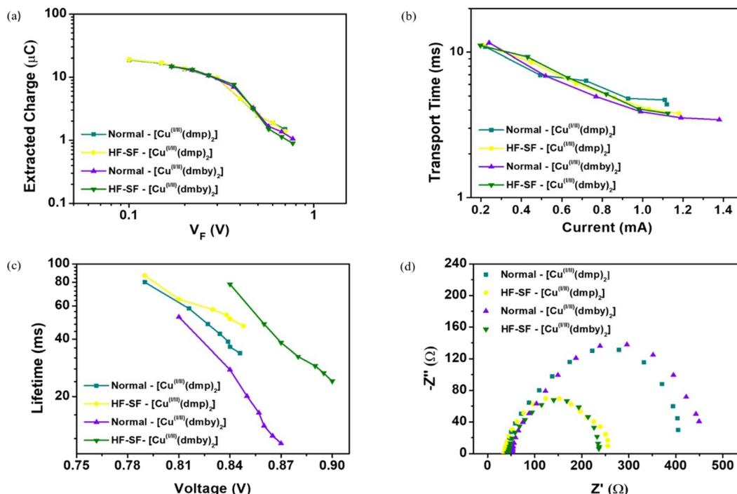
Fig. 2 (a) Charge extraction, (b) transport time (Toolbox), (c) lifetime (Toolbox), and (d) Nyquist plot (EIS) measurements for normal and HF-SF devices using  $[\text{Cu}^{(I/II)}(\text{dmp})_2]$  and  $[\text{Cu}^{(I/II)}(\text{dmby})_2]$  electrolytes.
