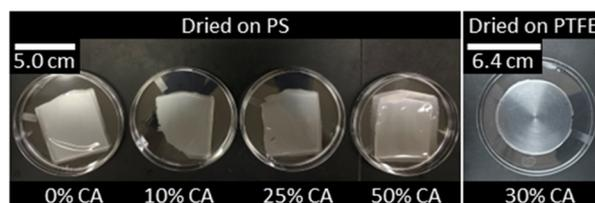
**Fig. 2** Photographs of CMC/CA films dried in polystyrene (PS) and polytetrafluoroethylene (PTFE) dishes.
