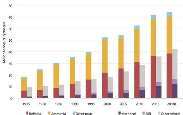
Fig. 1 World consumption of H<sub>2</sub> for different applications, ranging from ammonia manufacturing to direct reduction of iron ores (DRI). Refining is for petrochemicals, while methanol is an alternate fuel made using H<sub>2</sub>.<sup>6</sup> The world consumption has increased steadily from ~30 Mt in 1975 to 120 Mt in 2018 with refining and ammonia production being the major users.
