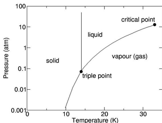
Fig. 3 Pressure–temperature or phase stability diagram for H<sub>2</sub> shows the temperature–pressure fields, where it exists as gas, liquid or solid. It can be seen that extremely low temperatures and high pressures will be required to transform from one phase to another, including the solid phase. There are several variants within the solid and liquid phases and these are not shown here for simplicity. At room temperature and atmospheric pressure, it exists in the gaseous state.
