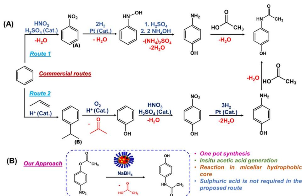
Fig. 7 (A) Commercial routes for acetaminophen synthesis. (B) Our approach for the direct synthesis of acetaminophen.
