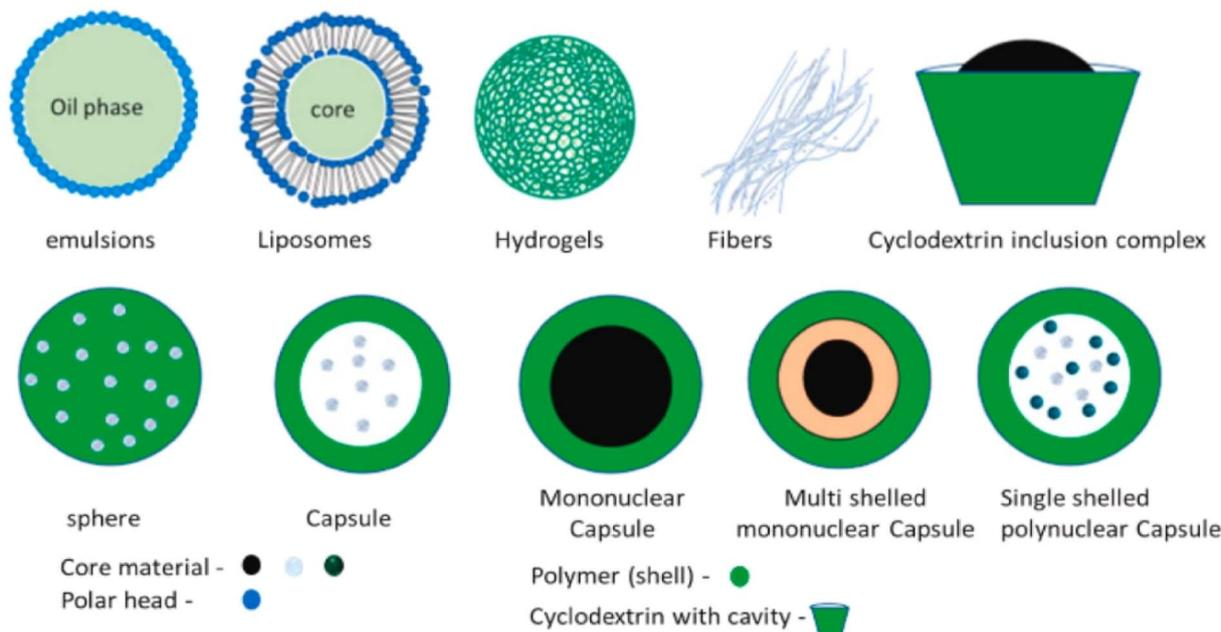
Fig. 6 Visual representation of encapsulated particle types.<sup>77</sup> Reprinted with permission from Elsevier (2023).
