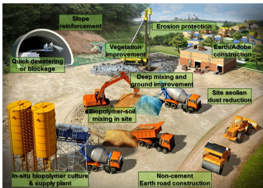
Fig. 10 Schematic representation of applications of biopolymers in the field of geotechnical engineering. 136 Reprinted with permission from Sustainability (2016).
