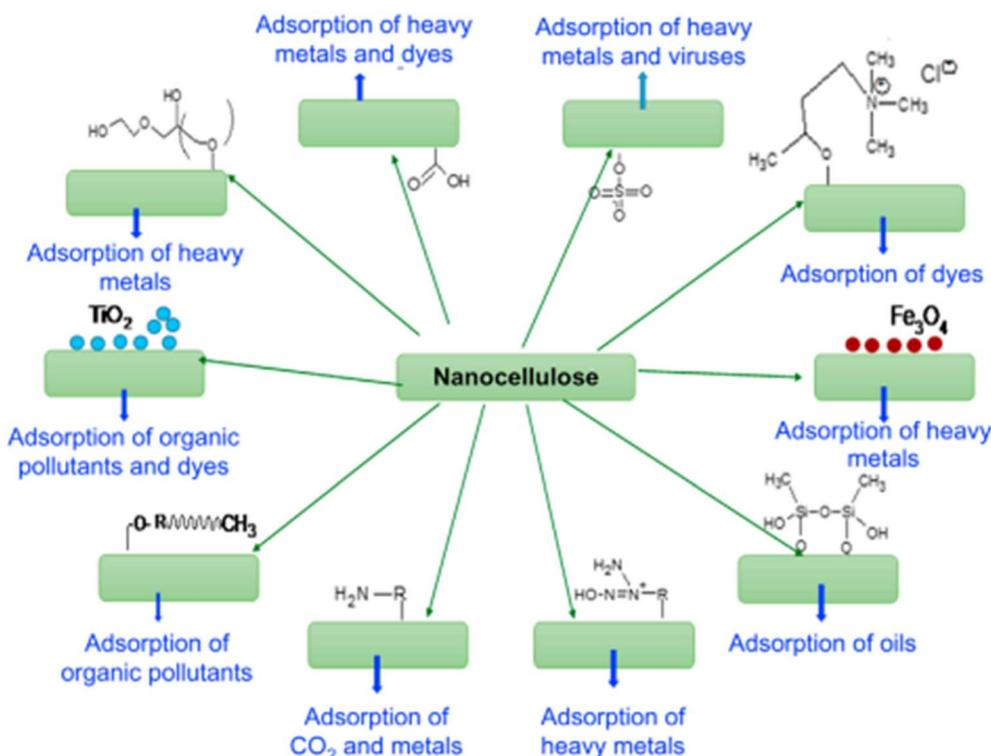
Fig. 8 Possible strategies for surface modification of nanocellulose according to the pollutant class.<sup>110</sup> Reprinted with permission from Woodhead Publishing Series (2017).
