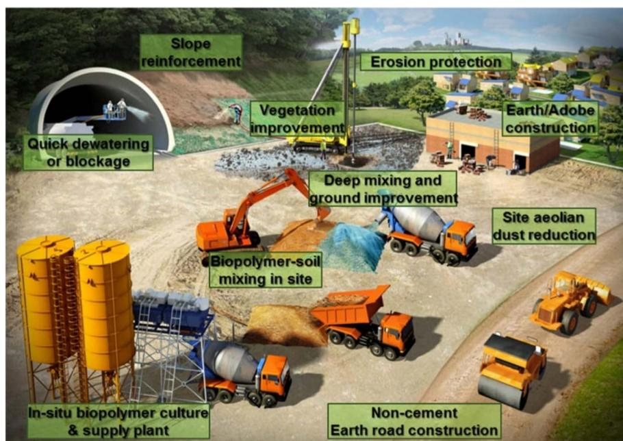
Fig. 10 Schematic representation of applications of biopolymers in the field of geotechnical engineering.<sup>136</sup> Reprinted with permission from Sustainability (2016).
