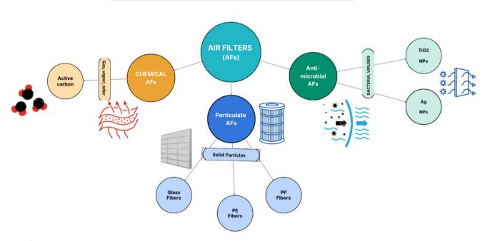
Fig. 12 Classification and types of the air filters that are currently deployed
