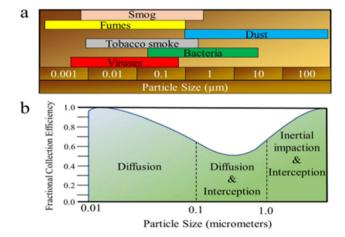
Fig. 15 (a) Size proportions of common air pollutants and (b) fractional collection effectiveness for various mechanical filters in relation to the contaminant diameter.<sup>150</sup> Reprinted with permission from ACS Publication (2021).
