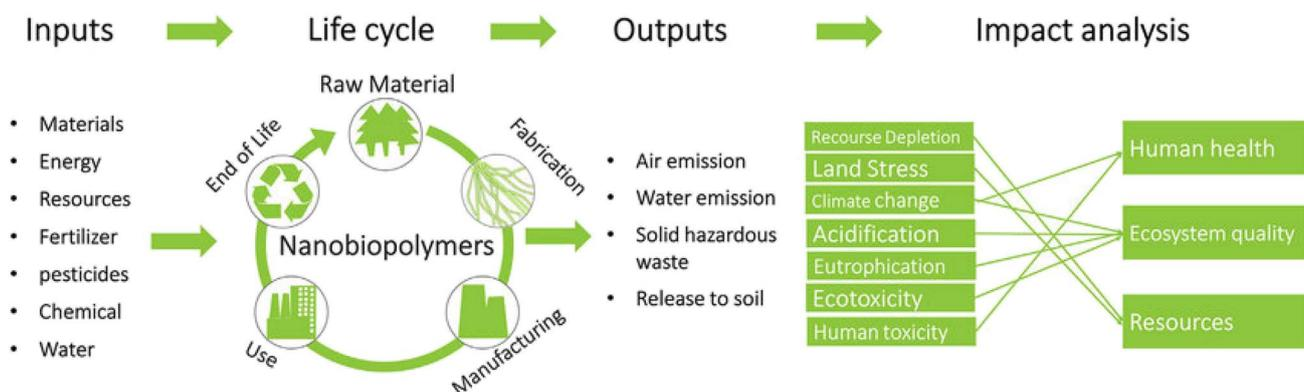
Fig. 1 Life cycle assessment for nanobiopolymers. Copyright (2018) Wiley. Used with permission from Nanobiopolymers Fabrication and Their Life Cycle Assessments.<sup>14</sup>
