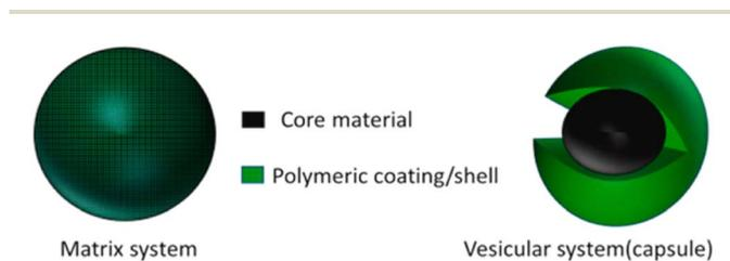
Fig. 5 Visual representation of encapsulation components.<sup>77</sup>
