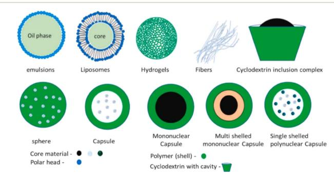
Visual representation of encapsulated particle types. 77 Reprinted with permission from Elsevier (2023).
