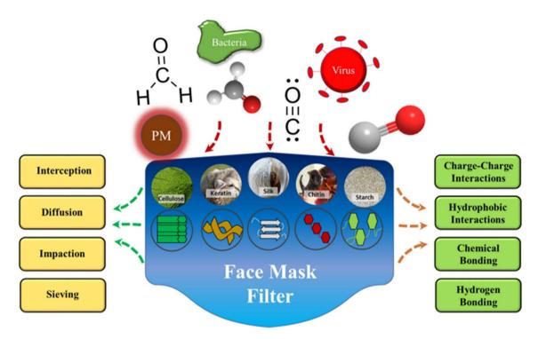
Fig. 13 Materials for biopolymer-based filtration made from various protein and polysaccharide sources. Particulate matter (PM), viruses, bacteria, and smoke pollutants can all be filtered out due to their particular surface chemistries and varied molecular interactions. Reprinted with permission from ACS Publication (2021).
