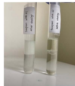
Fig. 4 Soapnut as an emulsifier: soapnut extract with oil after vigorous shaking and settling (left); water and oil after vigorous shaking and settling (right).
