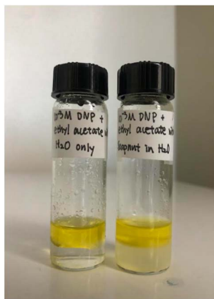
Fig. 9 A solution of dinitrophenyl hydrazine in ethyl acetate and water (left) & a solution of dinitrophenylhydrazine in ethyl acetate and soapnut extract in water (right).
