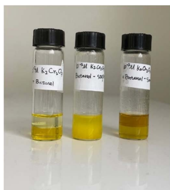
Fig. 7 Reverse micellar extraction of hexavalent chromium. Left: A mixture of K_2Cr_2O_7 in water with butanol. Middle: A mixture of K_2Cr_2O_7 in water with soapnut extract in butanol. Right: A mixture of K_2Cr_2O_7 in water (pH = 2) with soapnut in butanol.
