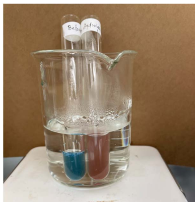
Fig. 6 Test for reducing sugars before hydrolysis and heating with Benedict's reagent (left) and after hydrolysis and heating with Benedict's reagent (right).
