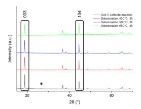
Fig. 2 Powder XRD patterns of cathode material (a) before treatment (black), (b) after delamination firing at 450 °C for 3 h (red), (c) after delamination firing at 500 °C for 3 h (blue) and (d) after delamination firing at 550 °C for 3 h (green). Carbon peaks are denoted by an asterisk (\*).
