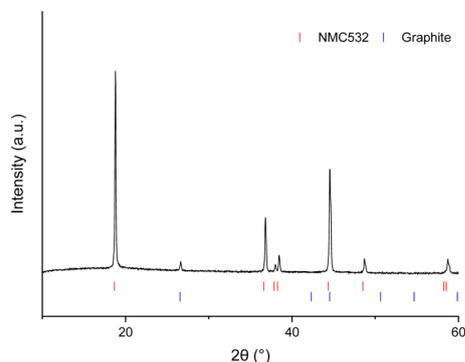
Fig. 1 Powder XRD patterns of cathode material with layered NMC oxide and carbon phases given as red and blue ticks respectively (CuK $\alpha_1$ /K $\alpha_2$ ). In these electrodes graphitic phase is used as a carbon additive.<sup>32</sup>
