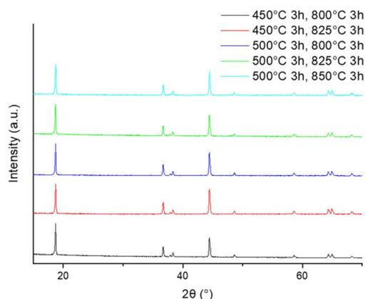
Fig. 3 XRD patterns of cathode material after two heat treatments (delamination: 450–550 °C for 3 h, final heat treatment 800–850 °C for 3 h in O<sub>2</sub>).
