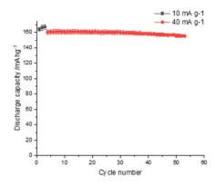
Fig. 8 Electrochemical data for relithiated sample (500 °C for 3 h in air followed by 825 °C for 3 h in  $O_2$  with 10 wt% LiOH·H<sub>2</sub>O) tested between the voltage range 2.5 and 4.3 V.
