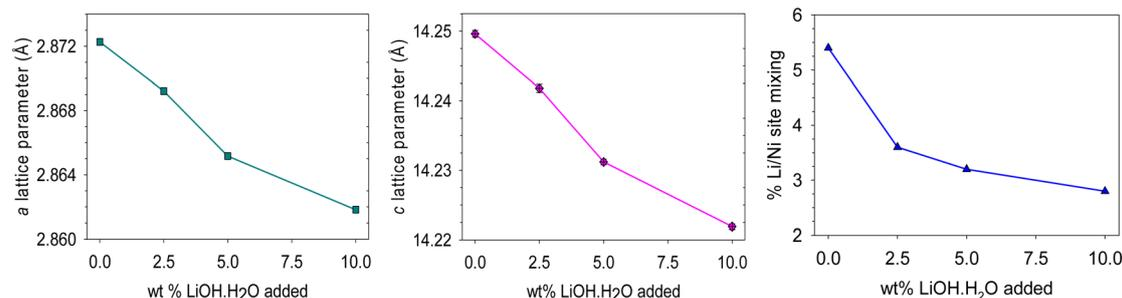
Fig. 4 Data from Rietveld refinement: lattice parameters (*a* and *c*) and % Li/Ni site mixing of relithiated cathode materials. Estimated errors are included, but are smaller than the symbols.
