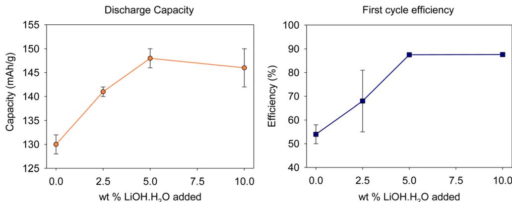
Fig. 6 Electrochemical data (discharge capacity (upper voltage limit 4.2 V) and first cycle efficiency) of relithiated cathode materials.
