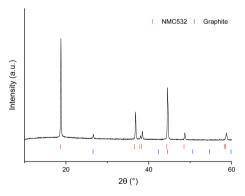
Fig. 1 Powder XRD patterns of cathode material with layered NMC oxide and carbon phases given as red and blue ticks respectively ( $\text{CuK}\alpha_1/\text{K}\alpha_2$ ). In these electrodes graphitic phase is used as a carbon additive.<sup>32</sup>
