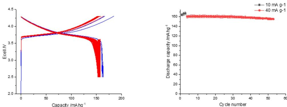
Fig. 8 Electrochemical data for relithiated sample (500 °C for 3 h in air followed by 825 °C for 3 h in O<sub>2</sub> with 10 wt% LiOH·H<sub>2</sub>O) tested between the voltage range 2.5 and 4.3 V.
