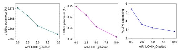
Fig. 4 Data from Rietveld refinement: lattice parameters (a and c) and % Li/Ni site mixing of relithiated cathode materials. Estimated errors are included, but are smaller than the symbols.
