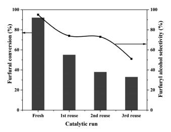
Fig. 3 Reusability of the 0.6%Pt/TiO<sub>2</sub> (C + R) catalyst. Reaction conditions: FF: 4.45 mmol; i-PrOH: 15 mL; temp: 30 °C; H<sub>2</sub>: 3 bar; substrate/metal molar ratio = 207; time: 3 h.
