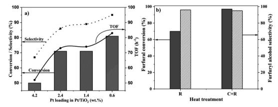
Fig. 2 (a) Effect of Pt loading on the catalytic activity for the liquid-phase hydrogenation of FF. Reaction conditions: FF: 4.45 mmol; i-PrOH: 15 mL; temp: 30 °C; H<sub>2</sub>: 3 bar; substrate/metal molar ratio = 207; time: 2 h. (b) Comparison of the catalytic data of 0.6%Pt/TiO<sub>2</sub> (C + R) and 0.6%Pt/TiO<sub>2</sub> (R) for the liquid phase hydrogenation of FF. Reaction conditions: FF: 4.45 mmol; i-PrOH: 15 mL; temp: 30 °C; H2: 3 bar; substrate/metal molar ratio = 207.
