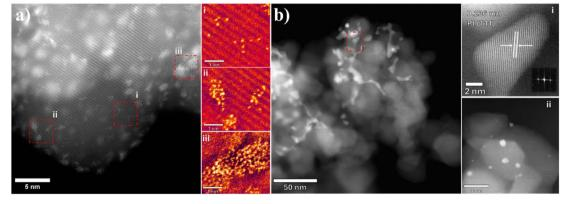
Fig. 5 Scanning transmission electron micrographs of (a) 4.2%Pt/TiO<sub>2</sub> (C + R) with the marked areas (i–iii) shown as high-pass filtered, coloured extracts to highlight the presence of single atoms, irregular clusters and rafts; (b) 4.2%Pt/TiO<sub>2</sub> (R) displaying large non-uniform corals with the marked area (i) showing the presence of Pt. Image ii shows the smaller more uniform nanoparticles also present.
