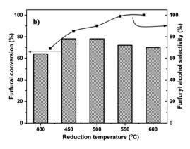
Fig. 1 Effect of heat treatment on 4.2%Pt/TiO2 for the liquid phase hydrogenation of furfural to furfural alcohol: (a) calcined-only (C) vs. reduction-only (R) vs. calcination + reduction (C + R) at 450 °C, time: 6 h; (b) catalytic data of 4.2%Pt/TiO<sub>2</sub> calcined at 450 °C followed by reduction at different temperatures. Reaction conditions: FF: 4.45 mmol; i-PrOH: 15 mL; temp: 30 °C; H<sub>2</sub>: 3 bar; substrate/metal molar ratio = 207; time: 3 h.
