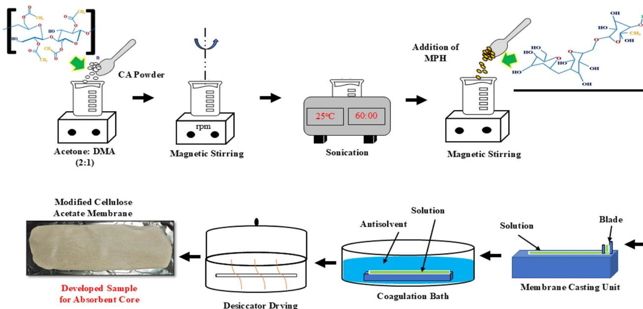
Scheme 2 Schematic illustration of modified cellulose acetate (MCA) membrane preparation using NIPS method.
