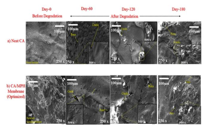
Fig. 14 SEM images of samples (before and after degradation): (a) neat CA; (b) MCA-2.
