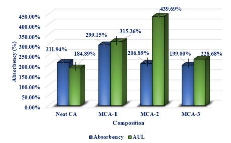
Fig. 5 A comparative study of free absorbency and absorbency under load at 60 min for neat CA and MCA-2 membrane samples.
