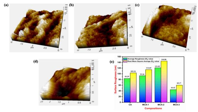
Fig. 10 AFM 3D images of (a) neat 5 wt% CA, (b) MCA-1, (c) MCA-2 and (d) MCA-3. (e) Graphical representation of average roughness (Ra) and root mean square roughness  $(R_a)$
