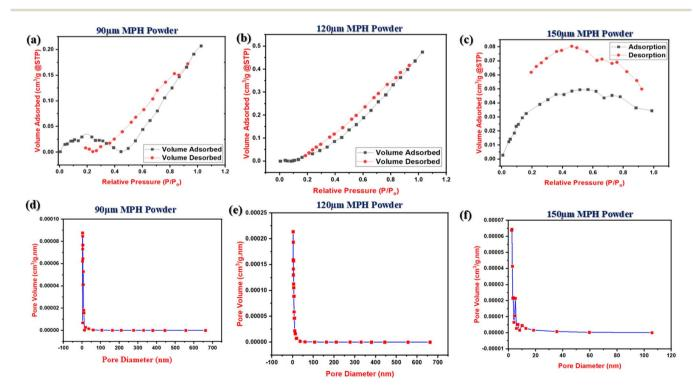
Fig. 2 (a-c) BET adsorption-desorption isotherms for 90 μm, 120 μm and 150 μm MPH powder respectively and (d-f) BJH pore size analysis of 90 μm, 120 μm and 150 μm MPH powder respectively.
