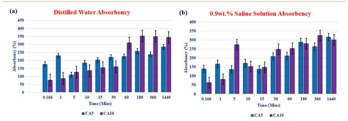
Fig. 3 Absorbency of neat cellulose acetate membrane samples at 5 wt% and 10 wt% in (a) distilled water and (b) 0.9 wt% saline solution.
