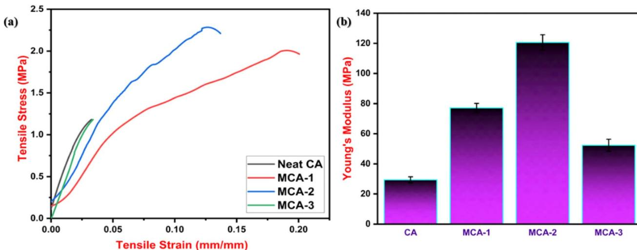
Fig. 11 (a) Tensile stress–tensile strain curves of (i) neat 5 wt% CA, (ii) MCA-1, (iii) MCA-2 and (iv) MCA-3. (b) Young's modulus value for all the compositions.
