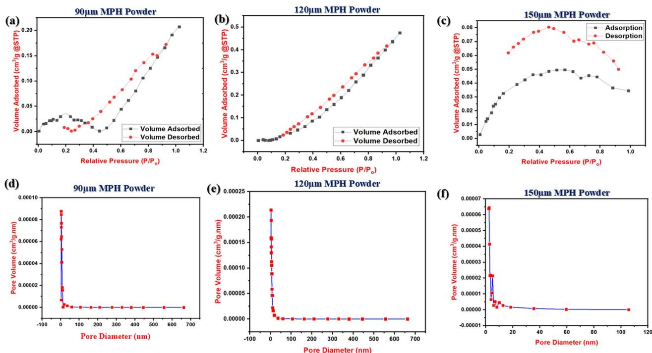
Fig. 2 (a–c) BET adsorption–desorption isotherms for 90  $\mu\text{m}$ , 120  $\mu\text{m}$  and 150  $\mu\text{m}$  MPH powder respectively and (d–f) BJH pore size analysis of 90  $\mu\text{m}$ , 120  $\mu\text{m}$  and 150  $\mu\text{m}$  MPH powder respectively.
