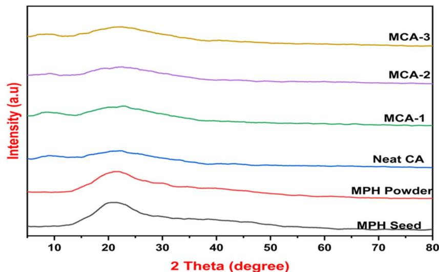
Fig. 6 XRD patterns of (i) *Mimosa pudica* seed, (ii) MPH powder, (iii) neat CA, (iv) MCA-1, (v) MCA-2, and (vi) MCA-3 samples.
