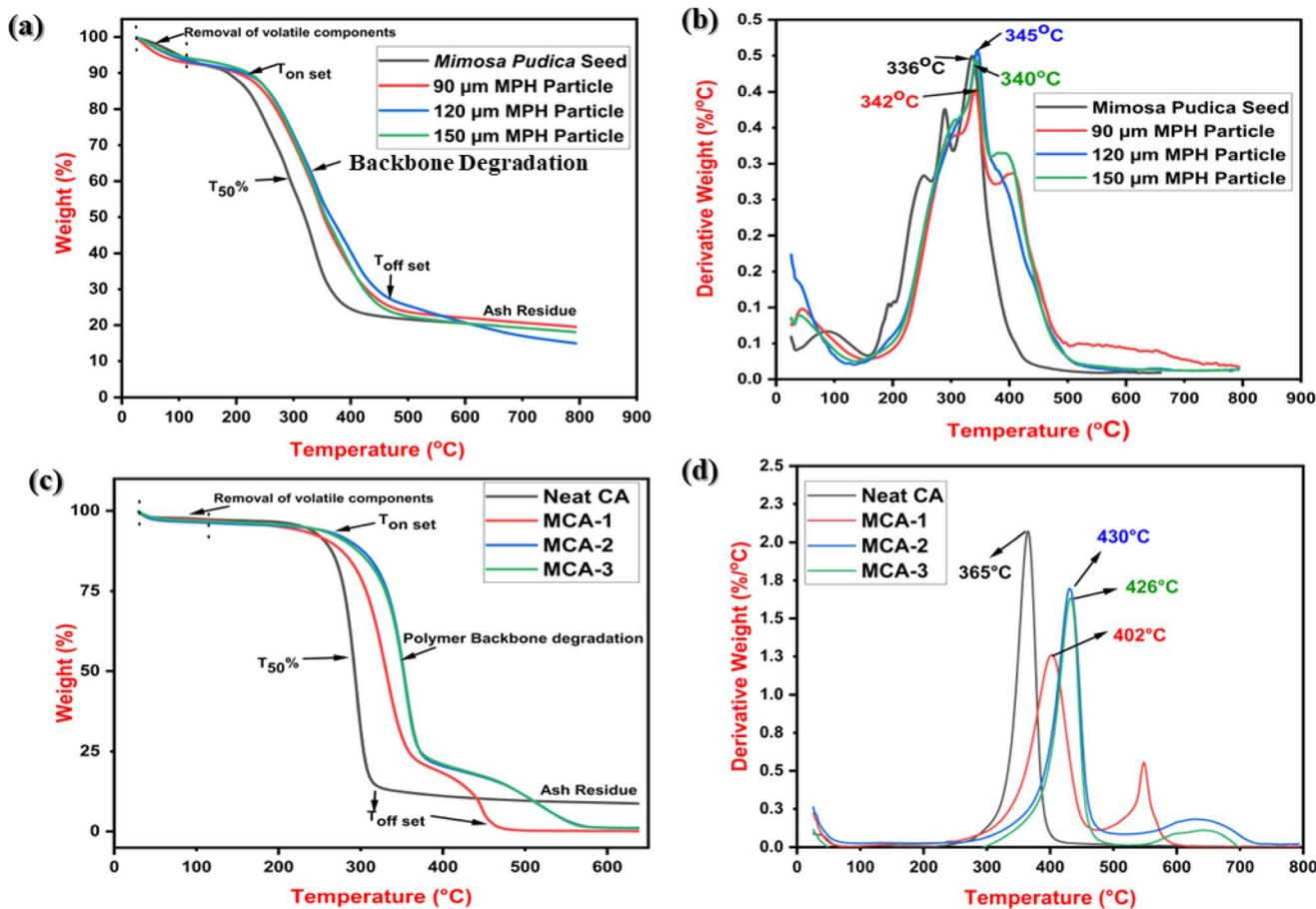
Fig. 12 (a) TGA thermograms for *Mimosa pudica* seed and 90–120 μm MPH powder. (b) Derivative thermograms (DTG). (c) TGA thermograms of (i) neat CA, (ii) MCA-1, (iii) MCA-2, (iv) MCA-3 and (d) DTG curves.
