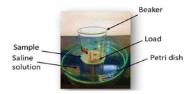
Scheme 3 Schematic illustration of an experimental setup for the AUL
