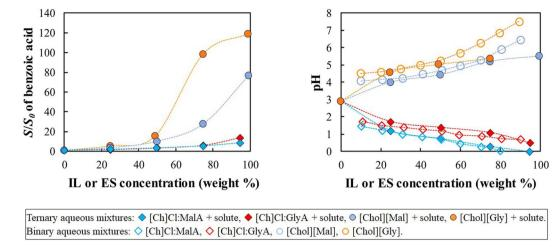
Fig. 2 (left plot) Relative solubility of benzoic acid, at 298.2 K, in aqueous solutions of [Ch]Cl:MalA, [Ch]Cl:GlvA, [Chol][Mal] and [Chol][Glv], (right plot) pH in ternary aqueous solutions, at 298.2 K, of [Ch]Cl:MalA + solute, [Ch]Cl:GlyA + solute, [Chol][Mal] + solute and [Chol][Gly] + solute; pH in binary aqueous solutions, at 303.2 K, of [Ch]Cl:MalA, [Ch]Cl:GlyA, [Chol][Mal] and [Chol][Gly]. Lines are a guide to the eyes.
