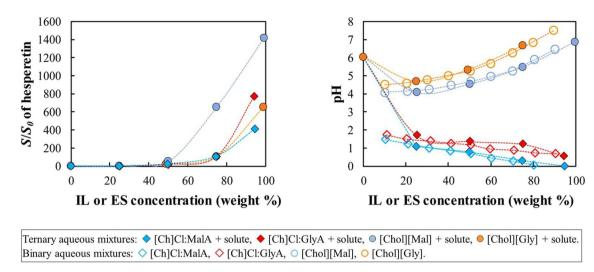
Fig. 4 (left plot) Relative solubility of (S)-hesperetin, at 298.2 K, in aqueous solutions of [Ch]Cl:MalA, [Ch]Cl:GlyA, [Chol][Mal] and [Chol][Gly]. (right plot) pH in ternary aqueous solutions, at 298.2 K, of [Ch]Cl:MalA + solute, [Ch]Cl:GlyA + solute, [Chol][Mal] + solute and [Chol][Gly] + solute; pH in binary aqueous solutions, at 303.2 K, of [Ch]Cl:MalA, [Ch]Cl:GlyA, [Chol][Mal] and [Chol][Gly]. Lines are a guide to the eyes.
