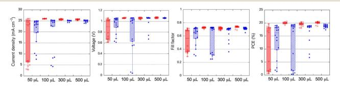
Fig. 6 Influence of anisole and chlorobenzene amount as antisolvent on the photovoltaic parameters of perovskite solar cells. The photovoltaic parameters are extracted from forward scan conditions, red (open dots) are for anisole and blue (square dots) for chlorobenzene.
