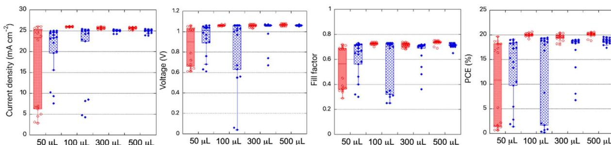
Fig. 6 Influence of anisole and chlorobenzene amount as antisolvent on the photovoltaic parameters of perovskite solar cells. The photovoltaic parameters are extracted from forward scan conditions, red (open dots) are for anisole and blue (square dots) for chlorobenzene.
