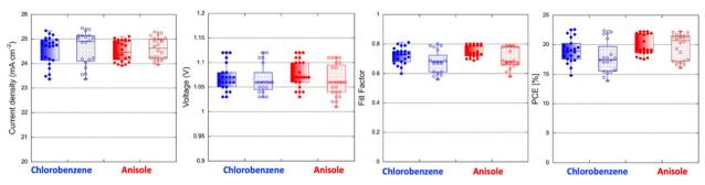
Fig. 3 Statistics of photovoltaic parameters (reverse scan full dots, forward scan open dots) of the perovskite solar cells,  $K_{0.025}(Cs_{0.1}-FA_{0.9})_{0.975}Pbl_3$  layer treated with chlorobenzene and anisole.
