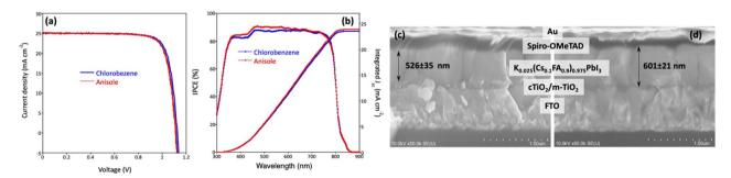
Fig. 4 (a) The best I-V curves (reverse and forward scans), and (b) IPCE of  $K_{0.025}(Cs_{0.1}FA_{0.9})_{0.975}Pbl_3$  based solar cells, perovskite layer treated with chlorobenzene and anisole, cross-sectional SEM images of  $K_{0.025}(Cs_{0.1}FA_{0.9})_{0.975}Pbl_3$  based solar cells, perovskite film treated by (c) chlorobenzene and (d) anisole.
