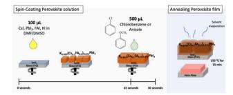
Fig. 1 Schematic representation of the processing method of  $K_{0.025}(Cs_{0.1}FA_{0.9})_{0.975}Pbl_3$  layer using chlorobenzene and anisole as antisolvents.
