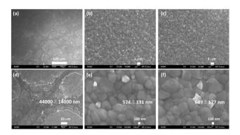
Fig. 2 SEM images on the surface of  $K_{0.025}(Cs_{0.1}FA_{0.9})_{0.975}Pbl_3$  film (a and d) without antisolvent treatment, (b and e) with chlorobenzene, and (c and f) with anisole (top (a–c) low-magnification and bottom (d–f) high-magnification SEM images).
