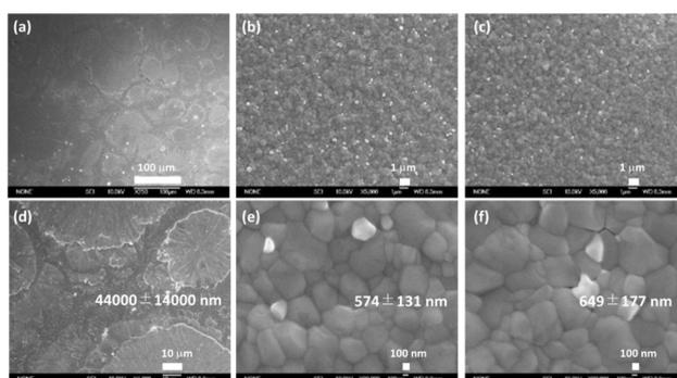
Fig. 2 SEM images on the surface of  $\text{K}_{0.025}(\text{Cs}_{0.1}\text{FA}_{0.9})_{0.975}\text{PbI}_3$  film (a and d) without antisolvent treatment, (b and e) with chlorobenzene, and (c and f) with anisole (top (a–c) low-magnification and bottom (d–f) high-magnification SEM images).
