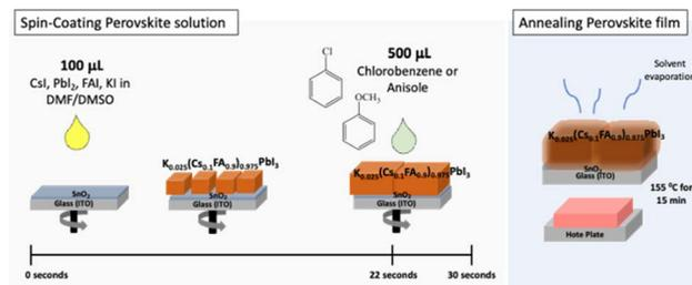
Fig. 1 Schematic representation of the processing method of  $\text{K}_{0.025}(\text{Cs}_{0.1}\text{FA}_{0.9})_{0.975}\text{PbI}_3$  layer using chlorobenzene and anisole as antisolvents.
