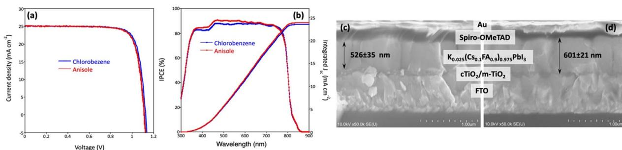
Fig. 4 (a) The best  $J$ - $V$  curves (reverse and forward scans), and (b) IPCE of  $K_{0.025}(Cs_{0.1}FA_{0.9})_{0.975}PbI_3$  based solar cells, perovskite layer treated with chlorobenzene and anisole, cross-sectional SEM images of  $K_{0.025}(Cs_{0.1}FA_{0.9})_{0.975}PbI_3$  based solar cells, perovskite film treated by (c) chlorobenzene and (d) anisole.
