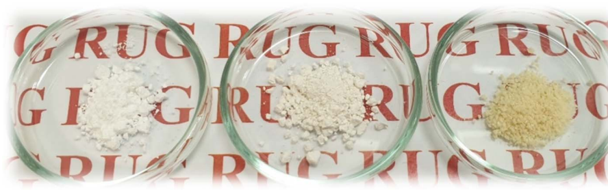
Fig. 4 From left to right, the products of poly(dodecamethylene-2,5-furanoate) synthesized with toluene from previous work, 34 p -cymene, and pinacolone.
