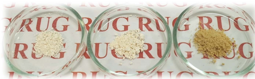
Fig. 8 From left to right: product appearance of P(2,5-FMF-co-2,5-DF) synthesized with toluene, p -cymene, and D -limonene.
