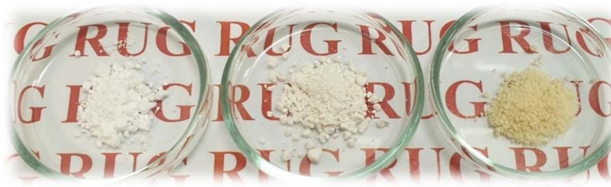
Fig. 4 From left to right, the products of poly(dodecamethylene-2,5-furanoate) synthesized with toluene from previous work,<sup>34</sup> *p*-cymene, and pinacolone.
