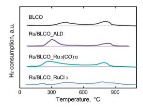
Fig. 3  $H_2$ -TPR profiles BLCO support, Ru/BLCO\_ALD, Ru/BLCO\_Ru $_3$ (CO) $_{12}$ , and Ru/BLCO\_RuCl $_3$ .
