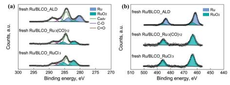
Fig. 2 XPS spectra of (a) C 1s + Ru 3d and (b) Ru 3p of Ru/BLCO\_ALD, fresh Ru/BLCO\_Ru<sub>3</sub>(CO)<sub>12</sub>, and fresh Ru/BLCO\_RuCl<sub>3</sub>.
