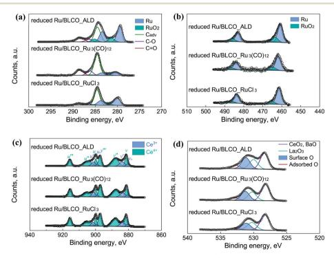
Fig. 6 XPS spectra of (a) C 1s + Ru 3d, (b) Ru 3p, (c) Ce 3d, and (d) O 1s of the reduced Ru/BLCO\_ALD, reduced Ru/BLCO\_RuGO\_12, and reduced Ru/BLCO\_RuGl3 catalysts.
