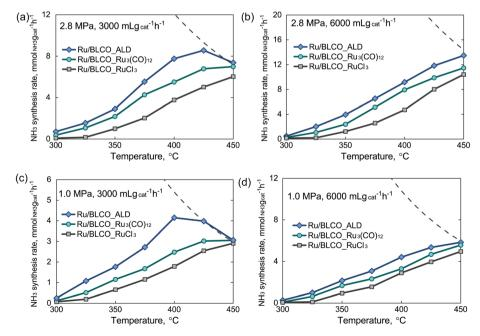
Fig. 7 Catalytic activities of ammonia synthesis using Ru/BLCO\_ALD, Ru/BLCO\_Ru<sub>3</sub>(CO)<sub>12</sub>, and Ru/BLCO\_RuCl<sub>3</sub> under different conditions: (a) 2.8 MPa and 3000 mL  $g_{cat}^{-1}h^{-1}$ , (b) 2.8 MPa and 6000 mL  $g_{cat}^{-1}h^{-1}$ , (c) 1.0 MPa and 3000 mL  $g_{cat}^{-1}h^{-1}$ , and (d) 1.0 MPa and 6000 mL  $g_{cat}^{-1}h^{-1}$ . Note: the dash line shows the equilibrium ammonia synthesis rate.
