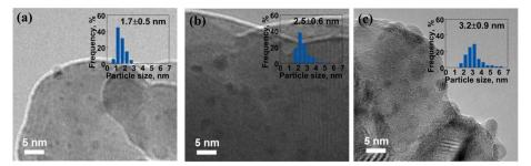
Fig. 5 TEM images of (a) reduced Ru/BLCO\_ALD, (b) reduced Ru/BLCO\_Ru<sub>3</sub>(CO)<sub>12</sub>, and (c) reduced Ru/BLCO\_RuCl<sub>3</sub> catalyst.
