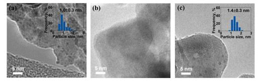
Fig. 1 TEM images of (a) fresh Ru/BLCO\_ALD, (b) fresh Ru/BLCO\_Ru<sub>3</sub>(CO)<sub>12</sub>, and (c) fresh Ru/BLCO\_RuCl<sub>3</sub>.
