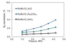
Fig. 8 Effects of pressure on the catalytic activities for ammonia synthesis using Ru/BLCO\_ALD, Ru/BLCO\_Ru<sub>3</sub>(CO)<sub>12</sub>, and Ru/BLCO\_RuCl<sub>3</sub> at 350 °C and 6000 mL  $g_{cat}^{-1}$  h<sup>-1</sup>.
