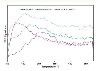
Fig. 4  $H_2$ -TPD profiles BLCO support, Ru/BLCO\_ALD, Ru/BLCO\_Ru<sub>3</sub>(CO)<sub>12</sub>, and Ru/BLCO\_RuCl<sub>3</sub>.
