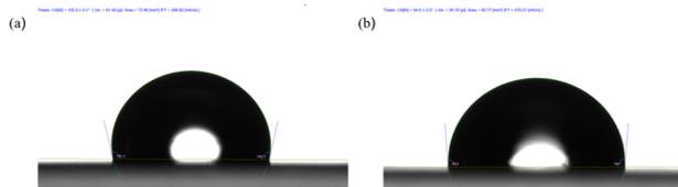
Fig. 10 Contact angle zinc foil (a) without additives; (b) with PI4.
