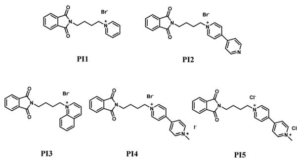
Fig. 1 Molecular structures of quaternary ammonium salts (**PI1–PI5**).
