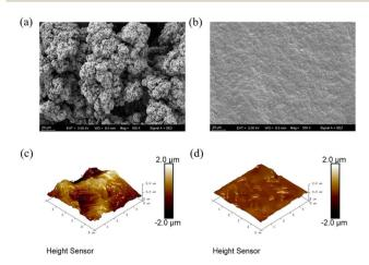
Fig. 8 (a and b) SEM images; (c and d) AFM images were obtained under the conditions of original electrolyte and PI4 electrolyte respectively at 1.5 A current for 30 min.
