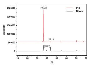
Fig. 9 XRD images were obtained under the conditions of the original electrolyte and PI4 electrolyte respectively at 1.5 A current for 30 min.
