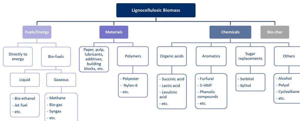
**Fig. 5** Lignocellulosic biomass valorisation products in one of the possible classifications showing the different end products, although many materials such as polymers are synthesised from chemicals, indicating the complexity of the lignocellulosic biomass valorisation process.
