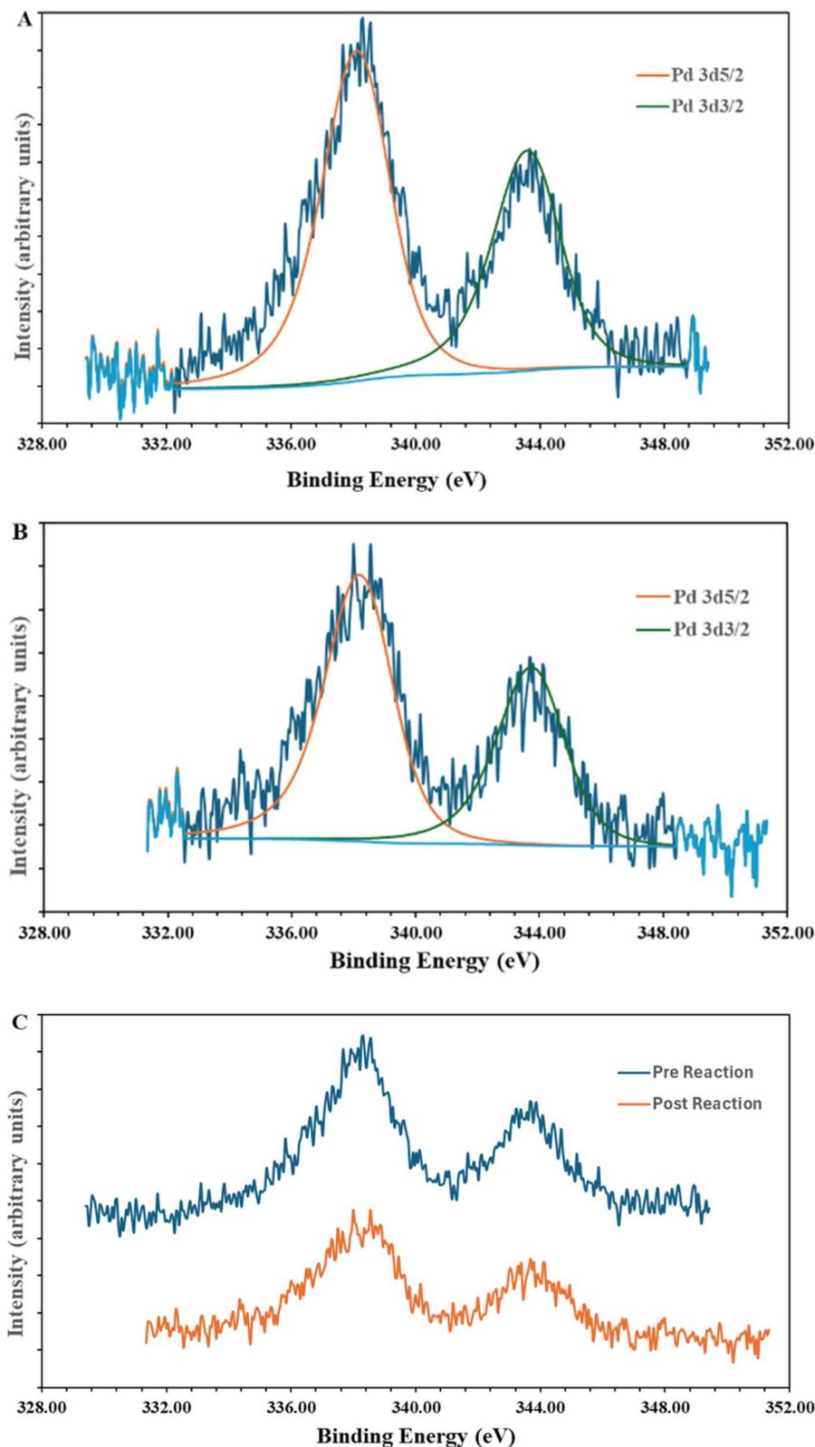
Fig. 4 XPS spectra of hybrid catalyst 2. (A) Catalyst as synthesized; (B) catalyst post catalytic reaction; (C) overlay XPS spectrum of as synthesized (pre) catalyst, and catalyst post catalytic reaction.
