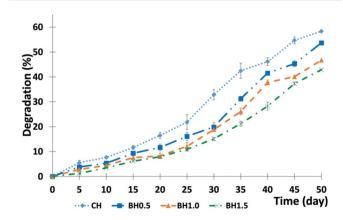
Fig. 8 Biodegradation rate of hydrogel composites in soil.
