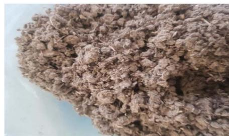
Fig. 4 Appearance of dewatered sludge (DS).
