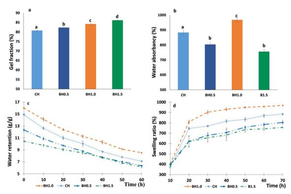
Fig. 7 Results of water retention studies and gel fraction. (a) Gel fraction (GF); (b) the water absorbency (WA); (c) the water retention ratio (WR) of de-swelling; (d) the swelling ratio (SR). Different letters on the bars show significant difference at 0.05 level.
