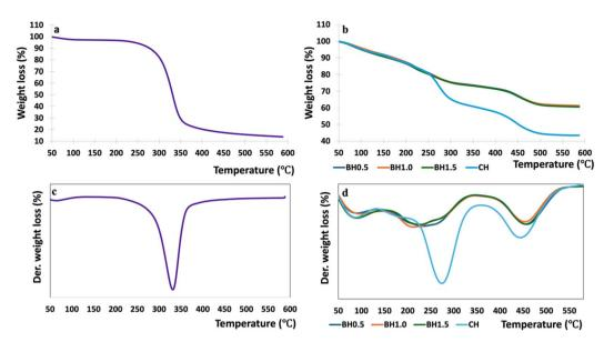
Fig. 6 Weight loss (a & b) and derivative weight loss (c & d) thermograms for the cellulose (a & c) and hydrogel composites (b & d) at various biochar content.
