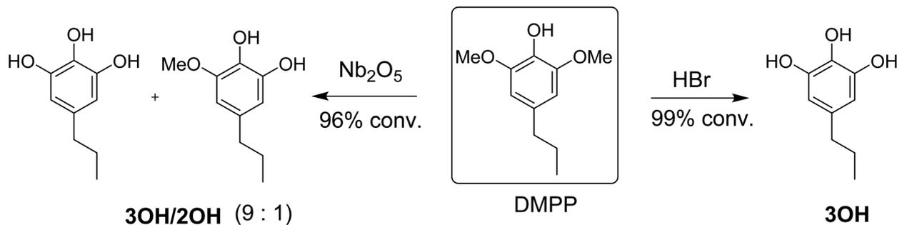
Scheme 1 Demethylation of DMPP via HBr to produce DMPPO (3OH) versus Nb<sub>2</sub>O<sub>5</sub> catalyzed reaction in water to make a mixture of DMPPO and DHEO (3OH/2OH) in 9 : 1 ratio.
