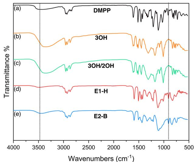
Fig. 4 FTIR spectra of (a) DMPP (b) 3OH (c) 3OH/2OH (d) E1-H (e) E2-B. The appearance and disappearance of the  $-OH$  band is highlighted at  $3331\text{ cm}^{-1}$  and the appearance of the epoxy band around  $927\text{ cm}^{-1}$  is highlighted.
