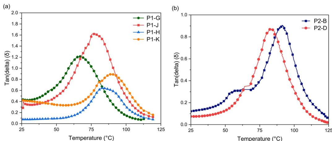
Fig. 7  $\tan(\delta)$  of (a) P1 and (b) P2 thermosets as a function of temperature. The ratio of the loss modulus ( $E''$ ) to the storage modulus ( $E'$ ) is defined as  $\tan(\delta)$ .  $T_g$  is the peak temperature in the  $\tan(\delta)$ .
