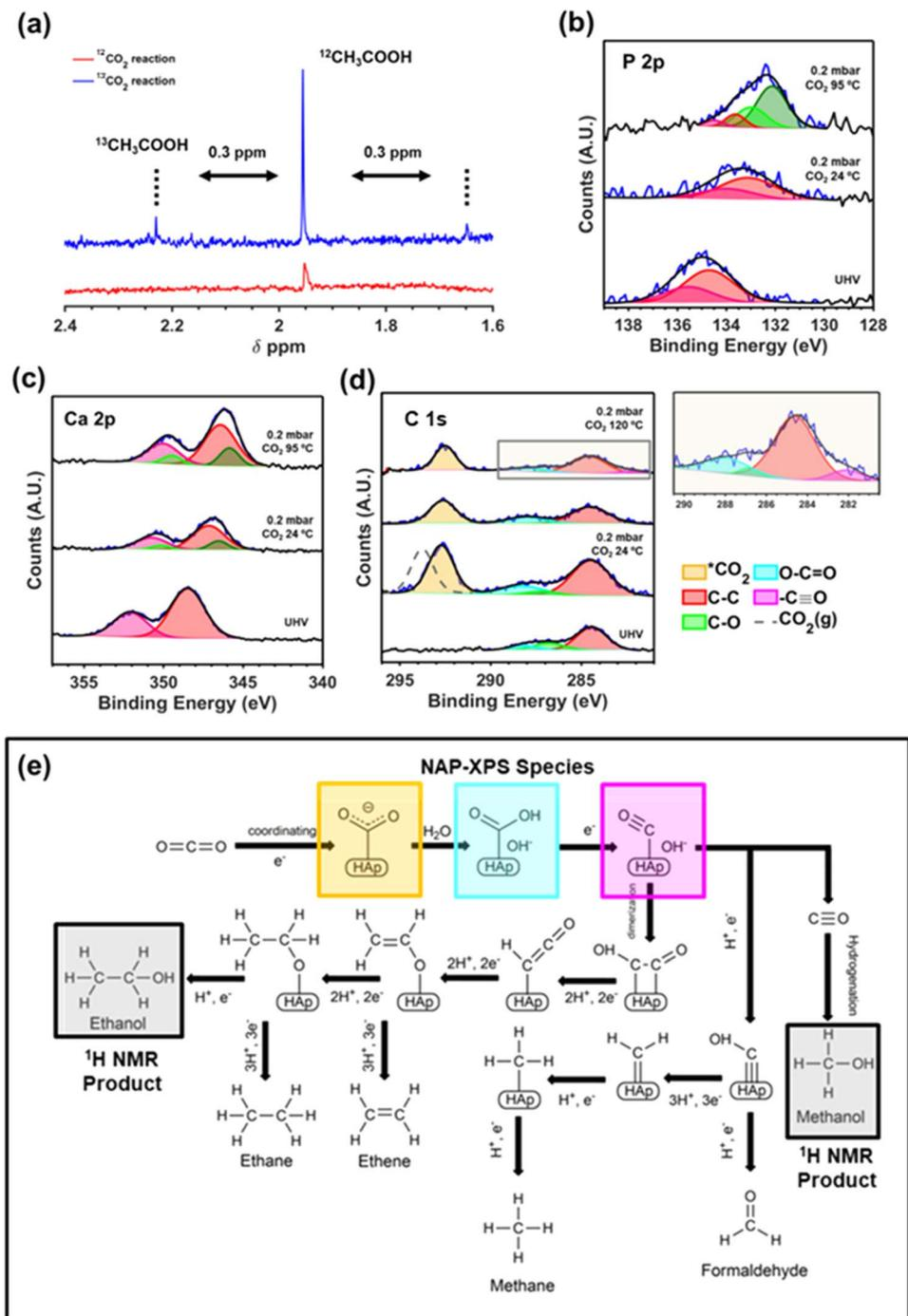
Fig. 4 (a) Isotope-labeling experiments. High resolution NAP-XPS studies using <sup>12</sup>CO<sub>2</sub> of the P 2p (b), Ca 2p (c) and C 1s (d). (e) Fixation mechanism derived from <sup>1</sup>H NMR and NAP XPS results.
