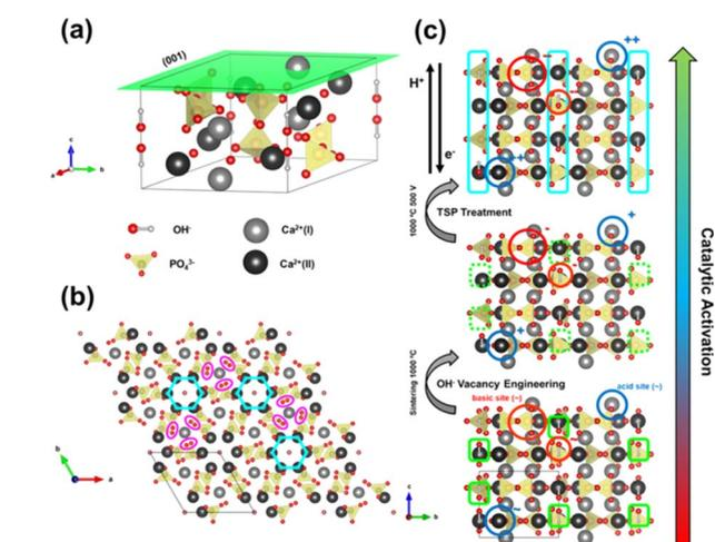
Scheme 1 Structure of HAP as a catalyst. (a) HAP unit cell  $P6_3/m$ . (b) (001) crystallographic plane observed from the *c*-axis direction. The  $\text{OH}^-$  channels and the Ca(i) 6-fold coordination are highlighted. (c) Structural changes and lattice refinement strategies adopted to achieve the catalytic activation of HAP.
