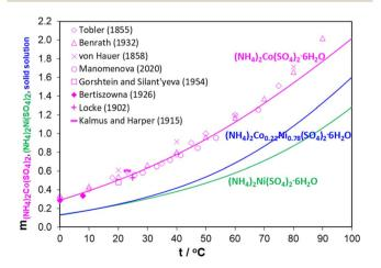
Fig. 2 Literature and calculated solubility of (NH<sub>4</sub>)<sub>2</sub>Co(SO<sub>4</sub>)<sub>2</sub>·6H<sub>2</sub>O<sub>4</sub>  $(NH_4)_2Ni(SO_4)_2 \cdot 6H_2O$ , and isolated Ni/Co Tutton's salt  $((NH_4)_2 - (NH_4)_2 -$  $Co_{0.22}Ni_{0.78}(SO_4)_2.6H_2O)$  in water as a function of solution temperature. Y-axis unit: mol salt per kg water.
