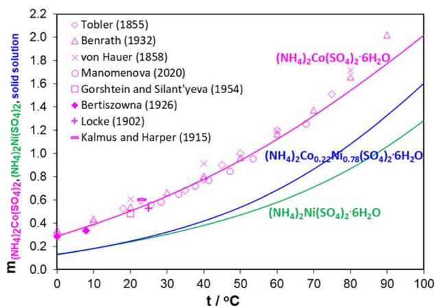
Fig. 2 Literature and calculated solubility of (NH<sub>4</sub>)<sub>2</sub>Co(SO<sub>4</sub>)<sub>2</sub>·6H<sub>2</sub>O, (NH<sub>4</sub>)<sub>2</sub>Ni(SO<sub>4</sub>)<sub>2</sub>·6H<sub>2</sub>O, and isolated Ni/Co Tutton's salt ((NH<sub>4</sub>)<sub>2</sub>Co<sub>0.22</sub>Ni<sub>0.78</sub>(SO<sub>4</sub>)<sub>2</sub>·6H<sub>2</sub>O) in water as a function of solution temperature. Y-axis unit: mol salt per kg water.
