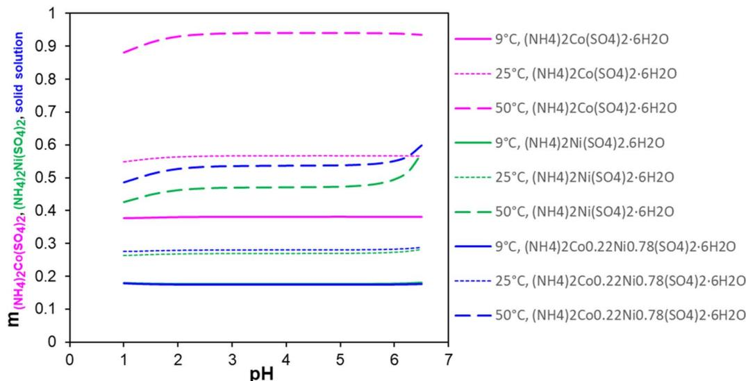
Fig. 3 Variations in the calculated solubilities of  $(\text{NH}_4)_2\text{Co}(\text{SO}_4)_2 \cdot 6\text{H}_2\text{O}$ ,  $(\text{NH}_4)_2\text{Ni}(\text{SO}_4)_2 \cdot 6\text{H}_2\text{O}$ , and Ni/Co Tutton's salt (referred to as solid solution, isolated  $(\text{NH}_4)_2\text{Co}_{0.22}\text{Ni}_{0.78}(\text{SO}_4)_2 \cdot 6\text{H}_2\text{O}$ ) in water as a function of solution pH at 9 °C, 25 °C and 50 °C. Y-axis unit: mol salt per kg water.
