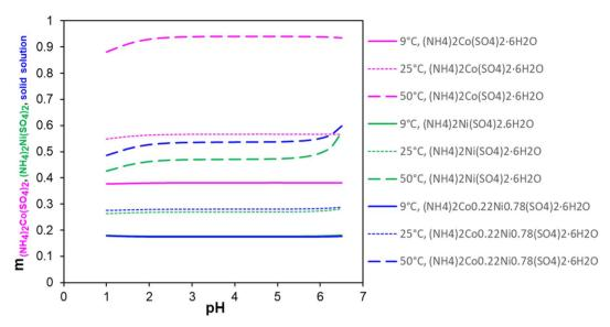
Fig. 3 Variations in the calculated solubilities of  $(NH_4)_2Co(SO_4)_2 \cdot 6H_2O$ ,  $(NH_4)_2Ni(SO_4)_2 \cdot 6H_2O$ , and Ni/Co Tutton's salt (referred to as solid solution, isolated  $(NH_4)_2Co_{0.22}Ni_{0.78}(SO_4)_2 \cdot 6H_2O$ ) in water as a function of solution pH at 9 °C, 25 °C and 50 °C. Y-axis unit: mol salt per kg water.
