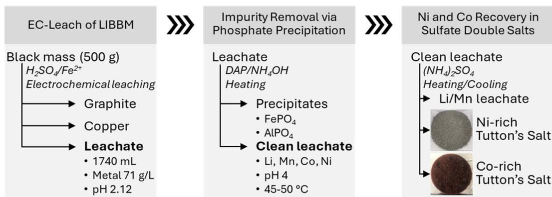
Fig. 7 LIBBM processing through three steps on the same leachate solution.
