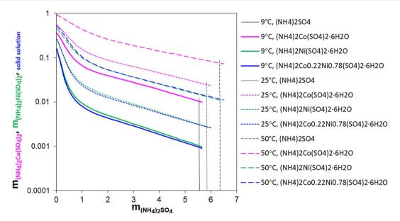
Fig. 4 Variation in calculated solubility of  $(NH_4)_2Co(SO_4)_2 \cdot 6H_2O$ ,  $(NH_4)_2Ni(SO_4)_2 \cdot 6H_2O$ , and Ni/Co Tutton's salt (referred to as solid solution, isolated  $(NH_4)_2Co_{0.22}Ni_{0.78}(SO_4)_2 \cdot 6H_2O$ ) in water as a function of added  $(NH_4)_2SO_4$  at 9 °C, 25 °C and 50 °C. Vertical black lines show the solubility of  $(NH_4)_2SO_4$  in this system at the specified temperatures. Unit: mol salt per kg water.
