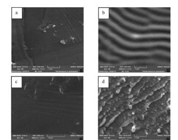
Fig. 4 SEM images of the surface and the cross section of the PVC film (a and c), and the 50% D2EHPA PIM (b and d). Reprinted with permission from Kazemi et al. (2021).46 Copyright 2021 Elsevier.
