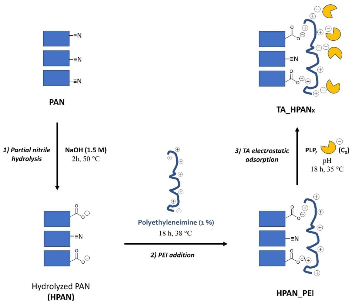
Fig. 1 Schematic representation of PAN functionalization and TA immobilization procedures, leading to TA\_HPAN<sub>xa</sub> or TA\_HPAN<sub>xb</sub>. In the case of TA\_HPAN<sub>2a</sub>, TA\_HPAN<sub>2b</sub>, TA\_HPAN<sub>3a</sub> and TA\_HPAN<sub>3b</sub>, an additional post-treatment was applied (with SA or GA, respectively) before the rinsing step.
