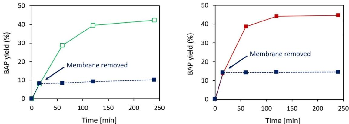
Fig. 8 Hot-filtration tests performed on TA\_HP3b (left) and TA\_PP3 (right), performed at equal immobilization concentration ( $C_0 = 0.25$  mg per mL TA, using TsRTA as TA). Full curves represent the standard catalytic tests while dotted curves represent the hot-filtration tests (*i.e.* in which the membrane-immobilized TAs were removed after 15 minutes). Reaction conditions: 10 mM rac-BMBA, 10 mM pyruvate, 1 mM PLP in 0.1 M HEPES pH 8 buffer, 37 °C (5 mL reaction volume).
