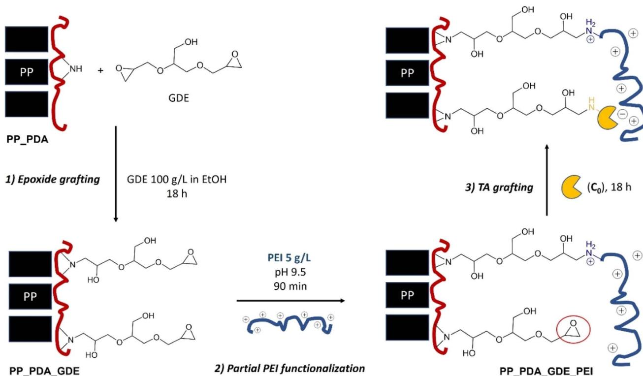
Fig. 2 Schematic representation of PP\_PDA functionalization and TA immobilization procedures on PP-based membranes, leading to TA\_PP catalysts. In some cases, the protocole was modified by adding an additional step (*i.e.* PLP immobilization) after the third step.
