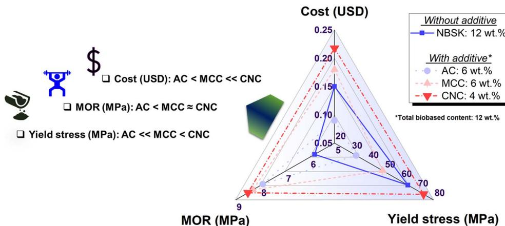
Fig. 5 Cost to performance ( $C/P$ ) analysis of fiber cement with micro-cellulosic additives (AC and MCC). Spider chart depicting the  $C/P$  (performance corresponds to yield stress and MOR). Note that the cost here refers to the total reinforcement/additive cost—it does not include the cost of other raw materials and processing. In the ESI, Table S11† has the detailed background information.
