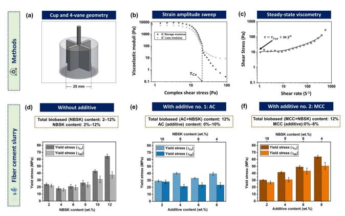
Fig. 2 Rheological characterization of the fiber cement slurry. (a) The cup and 4 vane rheometer geometry. Methods of computing yield stress using (b) the direct method—strain amplitude sweep, and (c) indirect method—steady state viscometry (Herschel—Buckley model). Reinforcing (NBSK) fiber/additive content dependent yield stress of the fiber cement slurry without additive, (d) NBSK; with micro-cellulosic additive, (e) AC (combination 1: AC and NBSK), and (f) MCC (combination 2: MCC and NBSK).
