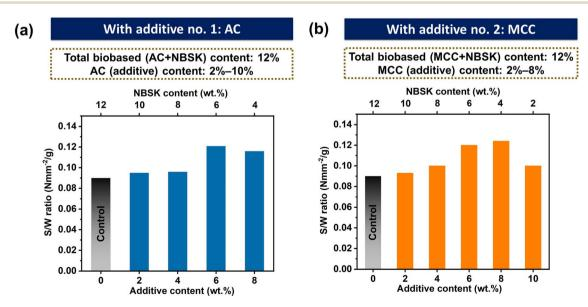
Fig. 4 Strength-to-weight (S/W) ratio analysis of fiber cement with micro-cellulosic additive (AC and MCC). (a) Combination 1 (AC and NBSK), (b) combination 2 (MCC and NBSK). Note that the ratio here refers to the mean modulus of rupture (MOR) values (in MPa) obtained from the threepoint bending test (vide supra) to the weight (g) of the specimen used for the mechanical characterization (Fig. 3). At MCC content of 10 wt%, the specimen cracked before curing (see Fig. S2†).
