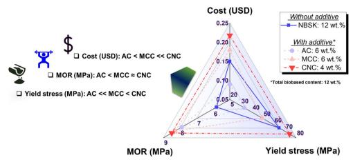
Fig. 5 Cost to performance (*C/P*) analysis of fiber cement with micro-cellulosic additives (AC and MCC). Spider chart depicting the *C/P* (performance corresponds to yield stress and MOR). Note that the cost here refers to the total reinforcement/additive cost—it does not include the cost of other raw materials and processing. In the ESI, Table S11† has the detailed background information.
