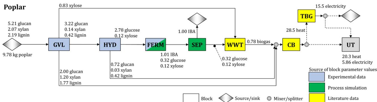
**Fig. 1** Block flow diagram of the baseline biomass-to-IBA biorefinery, using poplar as feedstock. Mass flows are in units of  $\text{kg kg}^{-1}$  of IBA produced, and heat and electricity flows are in units of  $\text{kWh kg}^{-1}$  of IBA. Abbreviations – CB: combustor and boiler, FERM: fermentation, GVL:  $\gamma$ -valerolactone, HYD: hydrolysis, SEP: separations, TBG: turbogenerator, UT: utilities, WWT: wastewater treatment.
