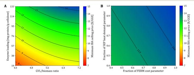
Fig. 3 MFSP of the biorefinery using sorghum as a function of (A) GVL/biomass mass ratio during pretreatment and enzyme loading during hydrolysis; and (B) cost parameter of FERM block and heat demand parameter of SEP block; the axis values are fractions of the base case parameter values.
