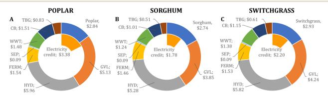
Fig. 2 Cost contributions in the baseline biorefinery using (A) poplar, (B) sorghum, and (C) switchgrass. Values shown are based on 1 GGE of IBA produced. The MFSP using each biomass is \$16.01, \$14.40, and \$15.55 GGE<sup>-1</sup> for poplar, sorghum, and switchgrass, respectively.
