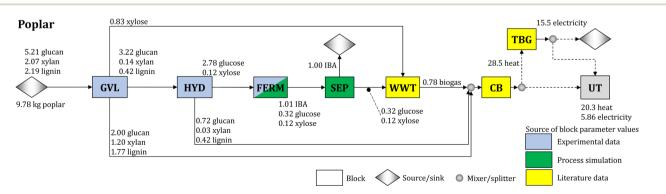
Fig. 1 Block flow diagram of the baseline biomass-to-IBA biorefinery, using poplar as feedstock. Mass flows are in units of kg kg<sup>-1</sup> of IBA produced, and heat and electricity flows are in units of kWh kg<sup>-1</sup> of IBA. Abbreviations – CB: combustor and boiler, FERM: fermentation, GVL:  $\gamma$ -valerolactone, HYD: hydrolysis, SEP: separations, TBG: turbogenerator, UT: utilities, WWT: wastewater treatment.
