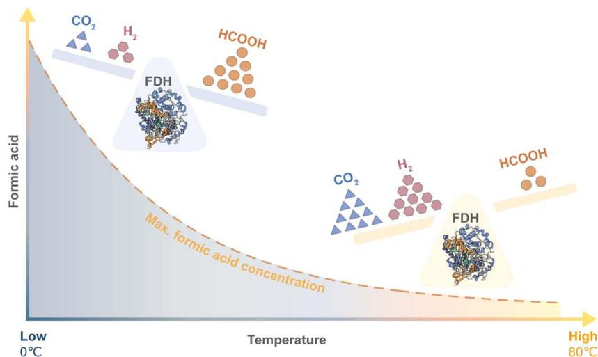
Fig. 4 Concentrations of dissolved formic acid in equilibrium with  $\text{CO}_2$  and hydrogen at different temperatures. At lower temperatures, the equilibrium favours formic acid formation, which in turn, creates a more acidic environment. But would require a catalyst that is able to operate at low temperatures, such as enzymes (FDH).
