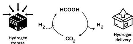
Fig. 2 Hydrogen presents a hazard for transportation. Instead, formic acid can easily store hydrogen, facilitating transport, and offering a viable H<sub>2</sub> delivery method. This occurs through a very convenient hydrogenation–dehydrogenation cycle.
