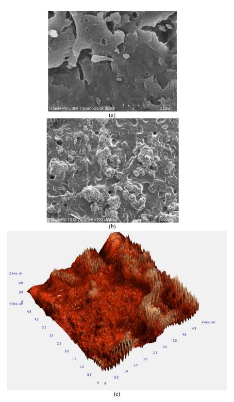
Fig. 1 FESEM images of (a) SG and (b) SG-PVP-poly(VSA) hydrogels; and AFM image of (c) SG-PVP-poly(VSA) hydrogels.
