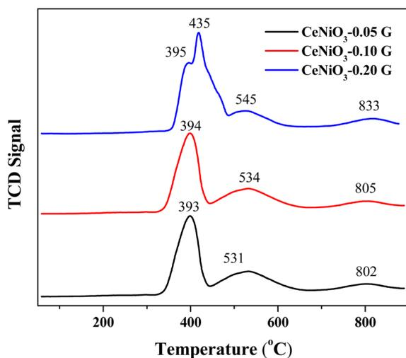
Fig. 3 H<sub>2</sub>-TPR profiles of CeNiO<sub>3</sub> perovskites obtained using different concentrations of gelatin.
