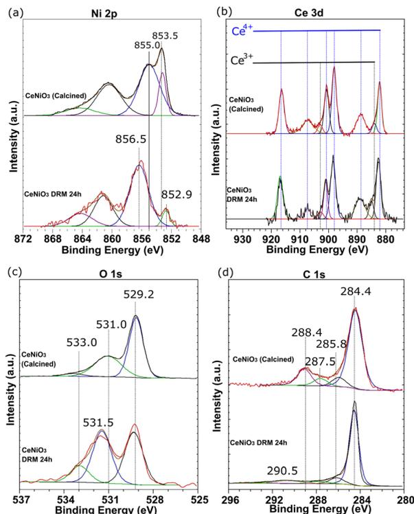
Fig. 6 XPS analysis of (a) Ni 2p, (b) Ce 3d, (c) O 1s, and (d) C 1s of CeNiO<sub>3</sub> (0.1 g gelatin) after calcination at 900 °C and the catalyst recovered from 24 h dry reforming at 600 °C.
