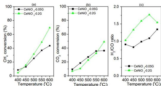
Fig. 8 Catalytic performance of CeNiO<sub>3</sub> perovskites at different temperatures: (a) CH<sub>4</sub> conversion; (b) CO<sub>2</sub> conversion; and (c) H<sub>2</sub>/CO ratios from CeNiO<sub>3</sub>-0.05G, CeNiO<sub>3</sub>-0.1G and CeNiO<sub>3</sub>-0.2G.
