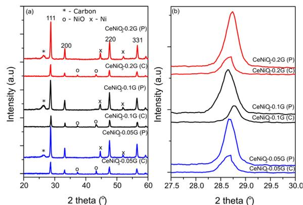
Fig. 1 XRD of  $CeNiO_3$  perovskite with (a) different concentrations of gelatin after calcination (C) and after the reaction (P); (b) changes in the high intense diffraction peak with different concentrations of gelatin before and after the reaction.
