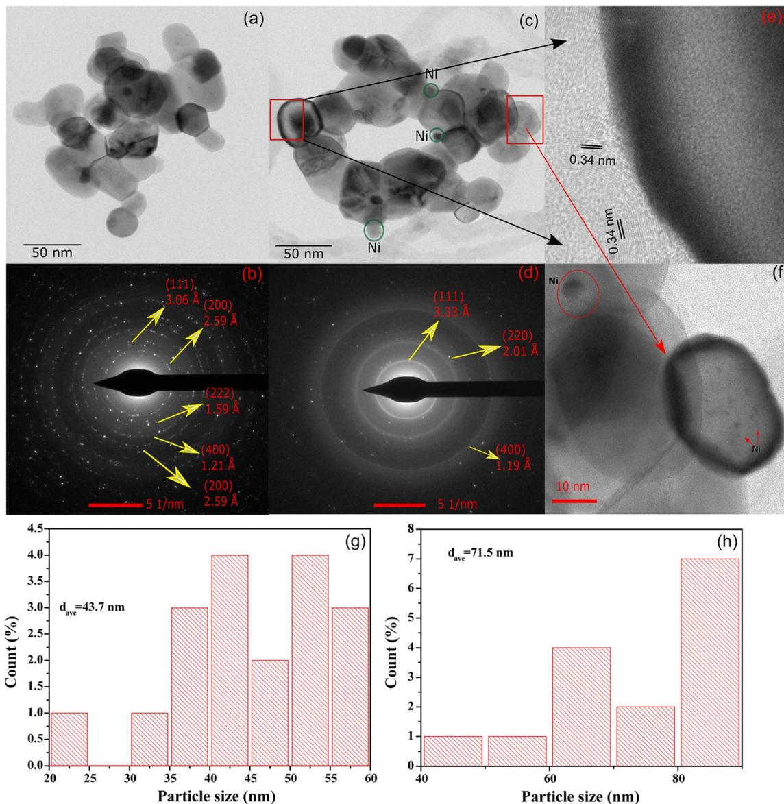
Fig. 5 HR-TEM images of (a) calcined CeNiO<sub>3</sub>-0.1G perovskite; (b) SAED pattern; (c) HR-TEM images of CeNiO<sub>3</sub> after DRM; (d) SAED pattern; (e) carbon nanotube on post-reaction CeNiO<sub>3</sub>; (f) Ni nanoparticles on CeO<sub>2</sub> after a 24 h reaction; (g) particle size distribution of CeNiO<sub>3</sub>-0.1G after calcination; and (h) particle size distribution of CeNiO<sub>3</sub>-0.1G after 24 h DRM reaction.
