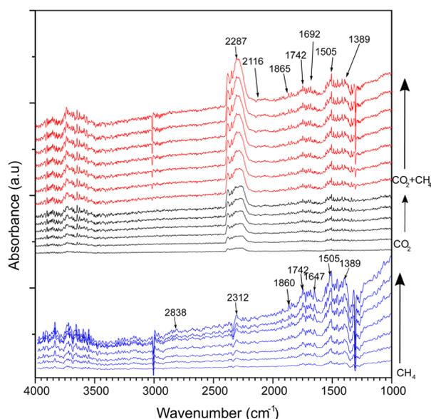
Fig. 9 In situ DRIFTS spectra of CeNiO<sub>3</sub> perovskite (0.2 g gelatin) under continuous flows of CH<sub>4</sub>, CO<sub>2</sub> and a mixture of CO<sub>2</sub> and CH<sub>4</sub> at 600 °C.
