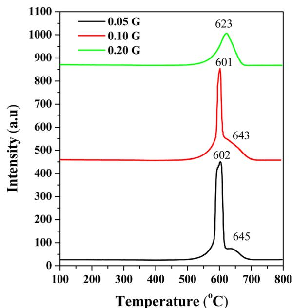
Fig. 4 TPO profiles of substituted CeNiO<sub>3</sub> perovskites synthesized using different concentrations of gelatin after a 24 h dry reforming reaction at 600 °C.
