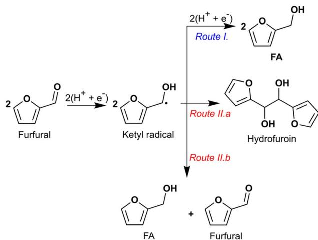
Scheme 2 Furfural conversion pathways to FA and hydrofuroin via a ketyl radical intermediate. It is proposed that route I is dominant on catalytic cathodes (e.g., Ru/ACC) where the ketyl radical is readily reduced to FA. Route II is dominant on non-catalytic cathodes (e.g., ACC) where a pair of ketyl radicals undergo dimerization (route II.a) to form hydrofuroin. Alternatively, a pair of ketyl radicals may undergo disproportionation (route II.b) to form FA and furfural.
