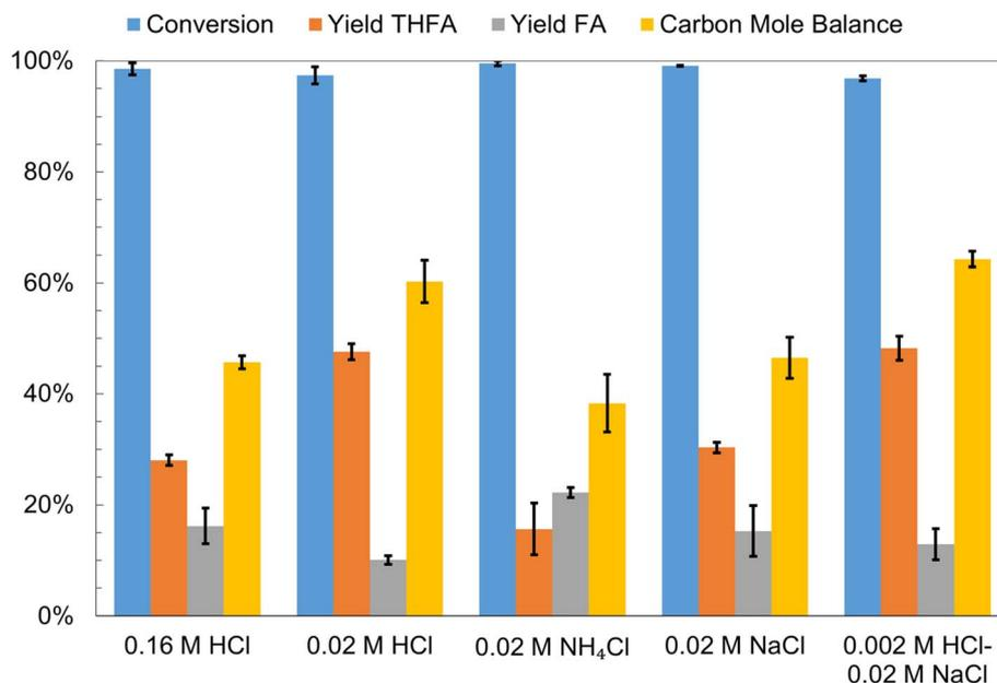
Fig. 7 ECH of furfural on Ru/ACC in different aqueous catholyte solutions. Experimental conditions: 0.02 M furfural, aqueous 0.16 M HCl, 0.02 M HCl, 0.02 M NH<sub>4</sub>Cl, 0.02 M NaCl and 0.002–0.02 M NaCl solutions (cathode compartment), 25 °C, 100 mA and 2 h. The corresponding anolyte solutions were composed of H<sub>3</sub>PO<sub>4</sub>, H<sub>3</sub>PO<sub>4</sub>, NH<sub>4</sub>Cl, NaCl and H<sub>3</sub>PO<sub>4</sub>. Error bars represent standard errors.
