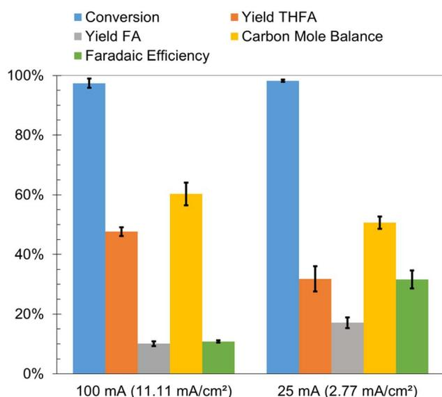
Fig. 8 ECH of furfural on Ru/ACC using different current densities (computed with respect to the geometric surface area). Experimental conditions: 0.02 M furfural; 0.02 M aqueous  $\text{HCl}$  solution (cathode compartment); 25 mA or 100 mA; 25 °C and 2 h. The reported faradaic efficiencies are computed with respect to the formation of FA and THFA. Error bars represent standard errors.
