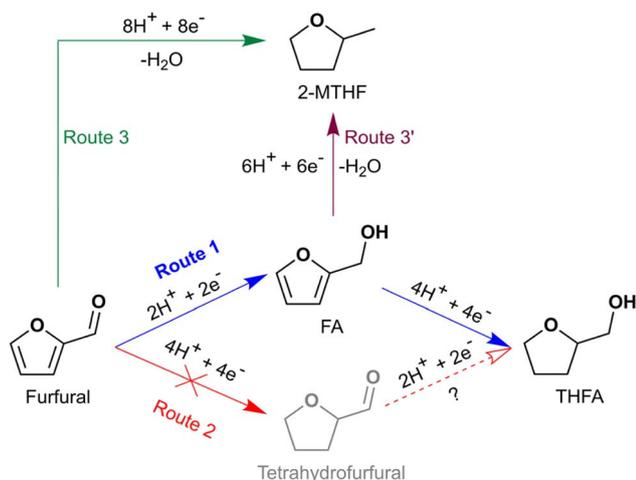
**Scheme 1** Summary of reactions observed during furfural ECH on Ru/ACC. Route 1 for THFA formation proceeds *via* hydrogenation of the formyl group, while route 2 proceeds *via* saturation of the heteroaromatic ring. Products not observed are depicted in grey. Transformation of tetrahydrofurfural to THFA by ECH was not investigated in the present study.
