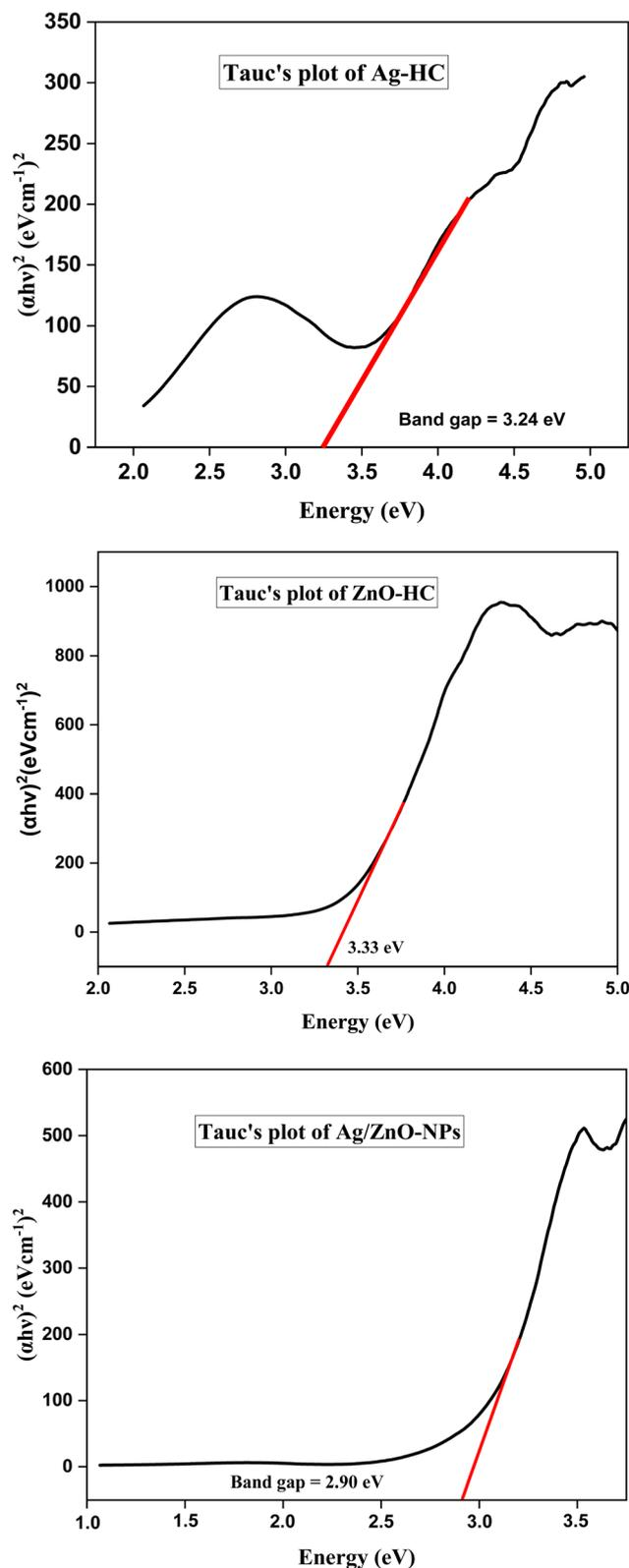
Fig. 4 Tauc plots of Ag-HC, ZnO-HC and Ag/ZnO-NPs.
