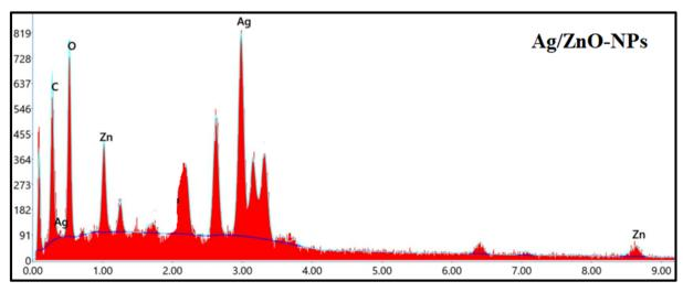
Fig. 8 EDX spectra of Ag-HC, ZnO-HC and Ag/ZnO-NPs.
