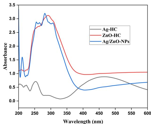
Fig. 3 UV-visible spectra of Ag-HC, ZnO-HC and Ag/ZnO-NPs.
