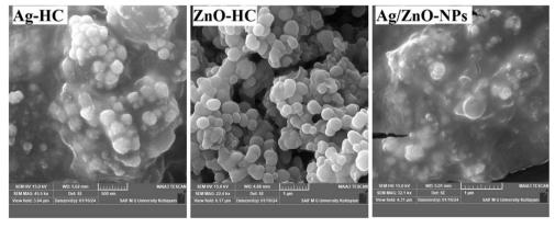
Fig. 7 FE-SEM images of Ag-HC, ZnO-HC and Ag/ZnO-NPs.
