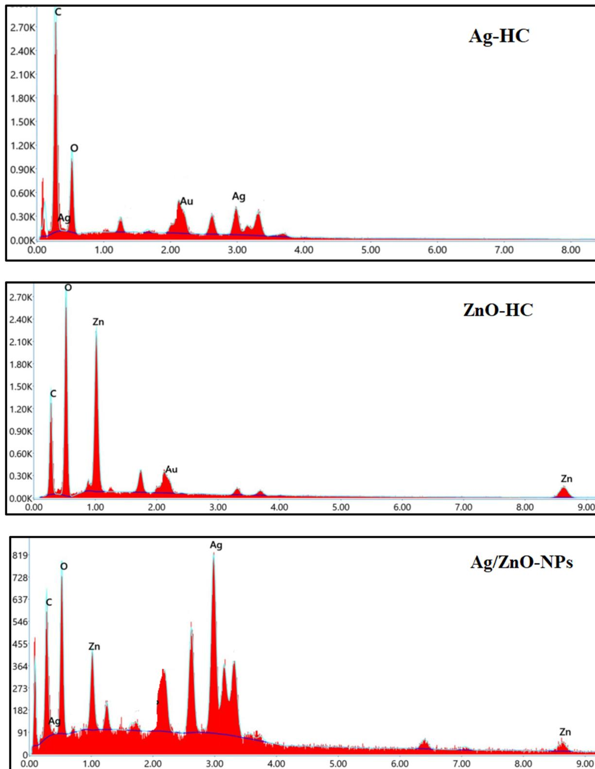
Fig. 8 EDX spectra of Ag-HC, ZnO-HC and Ag/ZnO-NPs.
