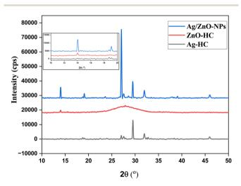
Fig. 6 XRD patterns of Ag-HC, ZnO-HC and Ag/ZnO-NPs. The inset shows the magnified XRD patterns of mono and bimetallic nanoparticles.
