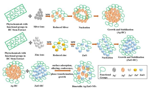
Scheme 2 Plausible mechanism involved in the formation of Ag-HC, ZnO-HC and Ag/ZnO-NPs.
