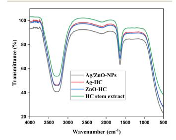
Fig. 5  $\,$  FT-IR spectra of HC stem extract, Ag-HC, ZnO-HC and Ag/ZnO-NPs.
