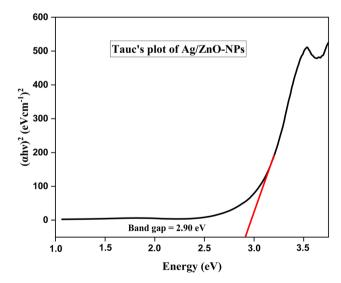
Fig. 4 Tauc plots of Ag-HC, ZnO-HC and Ag/ZnO-NPs.
