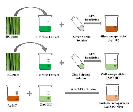
Scheme 1 Schematic representation of the formation of Ag-HC, ZnO-HC and Ag/ZnO-NPs
