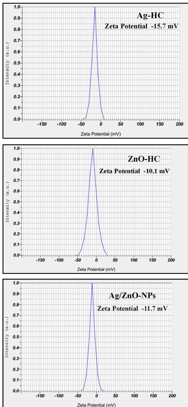
Fig. 10 Zeta potential graphs of Ag-HC, ZnO-HC and Ag/ZnO-NPs.
