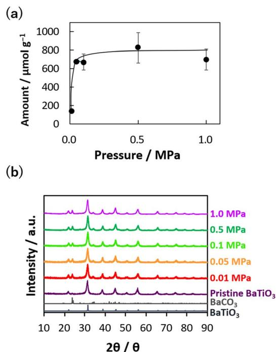
Fig. 1 (a) Weight increase of nanocatalysts after CO<sub>2</sub> thermolysis at 0.01–0.5 MPa. (b) XRD patterns of barium titanate nanocatalysts after CO<sub>2</sub> thermolysis. XRD patterns of barium carbonate and crystalline barium titanate are also shown as references.
