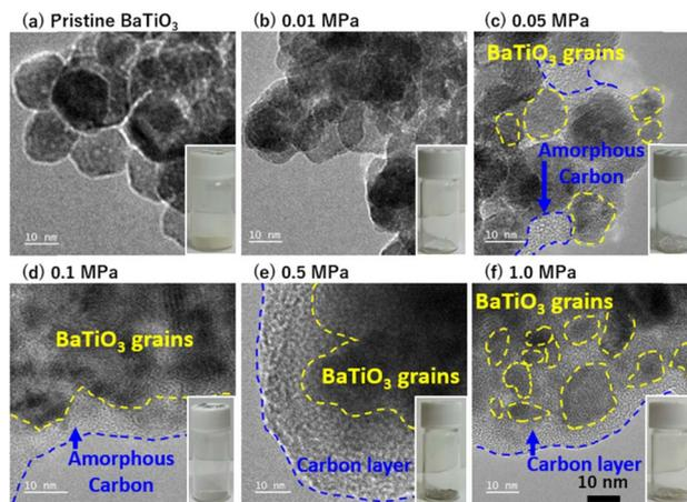
Fig. 3 TEM images of (a) pristine nanocatalyst and nanocatalyst after  $\text{CO}_2$  thermolysis at (b)  $0.01$ , (c)  $0.05$ , (d)  $0.1$ , (e)  $0.5$ , and (f)  $1.0$  MPa. The insets show the optical images of the nanocatalysts.
