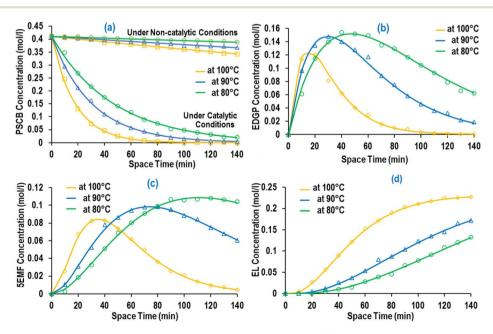
Fig. 9 (a) PSCB (under catalytic and non-catalytic conditions), (b) EDGP, (c) 5EMF and (d) EL concentrations at different reaction temperatures [line: predicted yield; marker: actual yield].
