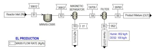
Fig. 11 Simulated process flow diagram of the EL PRODUCTION hierarchy block.
