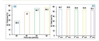
Fig. 7 (a) Effect of feed flow rate on EL yield. (b) DES2 reusability study in the MWVIS-CSSR.
