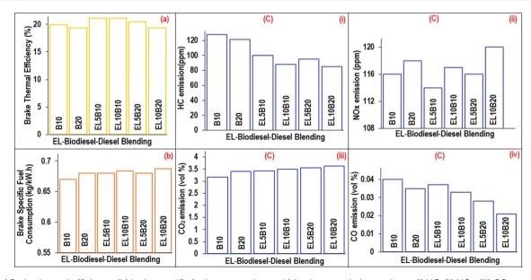
Fig. 15 (a) Brake thermal efficiency, (b) brake specific fuel consumption and (c) exhaust emission analyses: (i) HC, (ii) NO<sub>x</sub>, (iii) CO<sub>2</sub>, and (iv) CO of different blends
