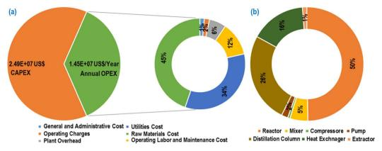
Fig. 14 (a) Total CAPEX and annual OPEX of the SCB to EL synthesis process. (b) Share of major equipment in the total equipment costs.
