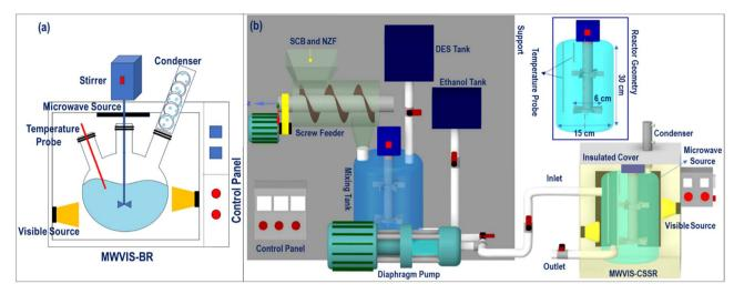
Fig. 2 (a) Batch EL synthesis in the MWVIS-BR; (b) continuous EL synthesis process in the MWVIS-CSSR.
