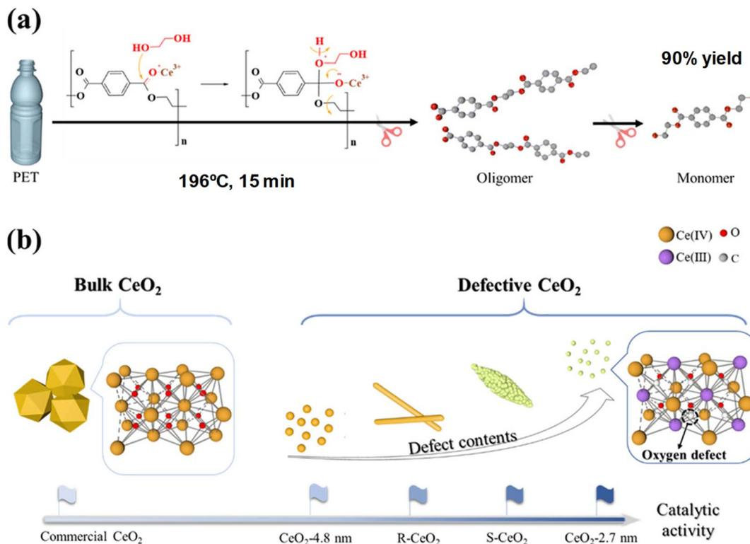
Scheme 15 (a) PET glycolysis (196 °C, 15 min) procedure over defective CeO<sub>2</sub> NPs. (b) Structures and catalytic activities of CeO<sub>2</sub> NPs with different morphologies. Reproduced with permission of ref. 56. Copyright (2022) American Chemical Society.
