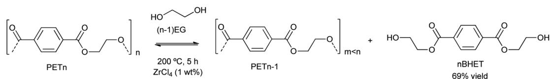
**Scheme 2** PET degradation by glycolysis into BHET using metal chlorides, *i.e.* ZrCl<sub>4</sub> (1% wt), at 200 °C during 5 h.
