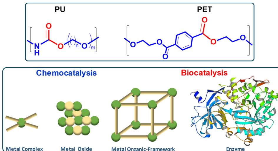
**Scheme 1** Similarities and differences between PU and PET condensation polymers reviewed here (top). Discrete metal ions, organometallic complexes, metal oxides and porous metal–organic frameworks as chemocatalysts vs. enzyme biocatalysts (bottom).
