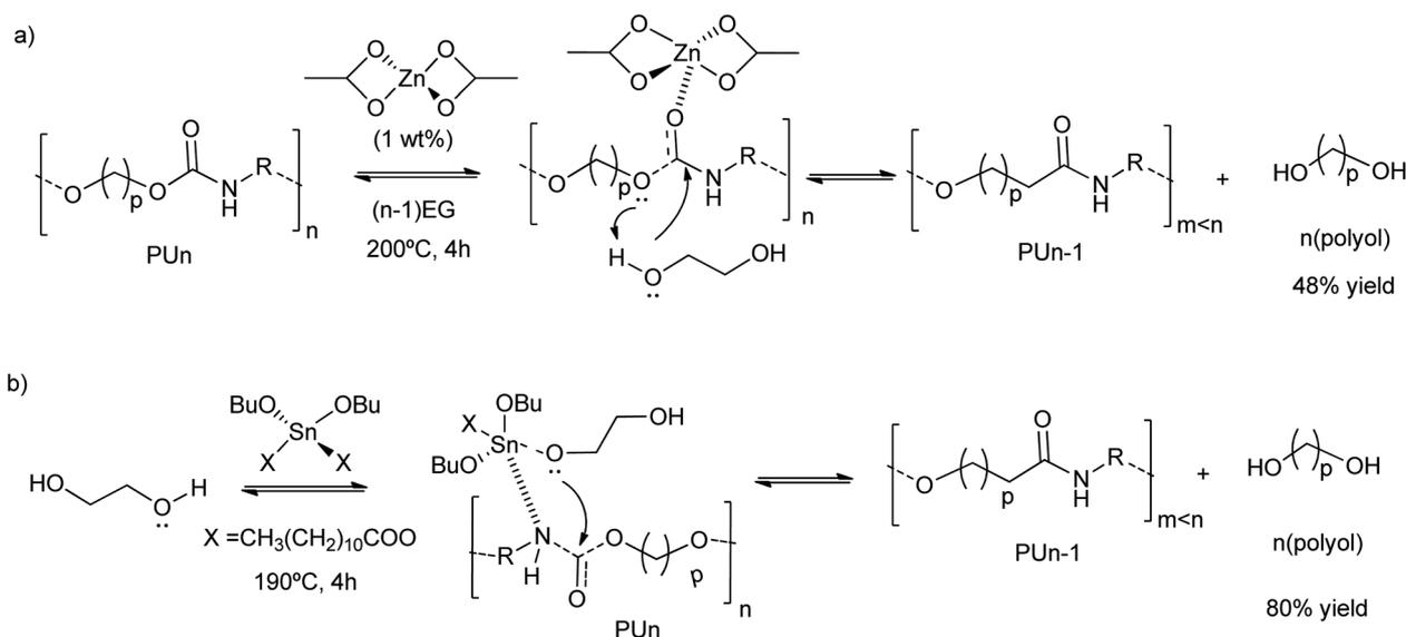
Scheme 5 Proposed mechanisms for PU degradation using Zn(OAc)<sub>2</sub> (a) or Sn(OBu)<sub>2</sub>X<sub>2</sub> (b) as a catalyst at 190–200 °C for 4 h.
