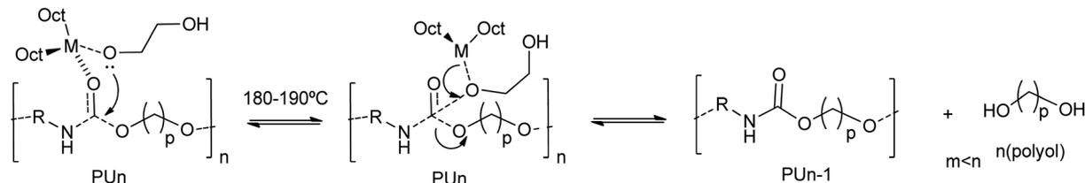
Scheme 6 Proposed mechanisms for PU degradation at 180–190 °C using octoate salts of metals (M = Li, Na, K, Sr, Co, Ni, Zn) as a catalyst.
