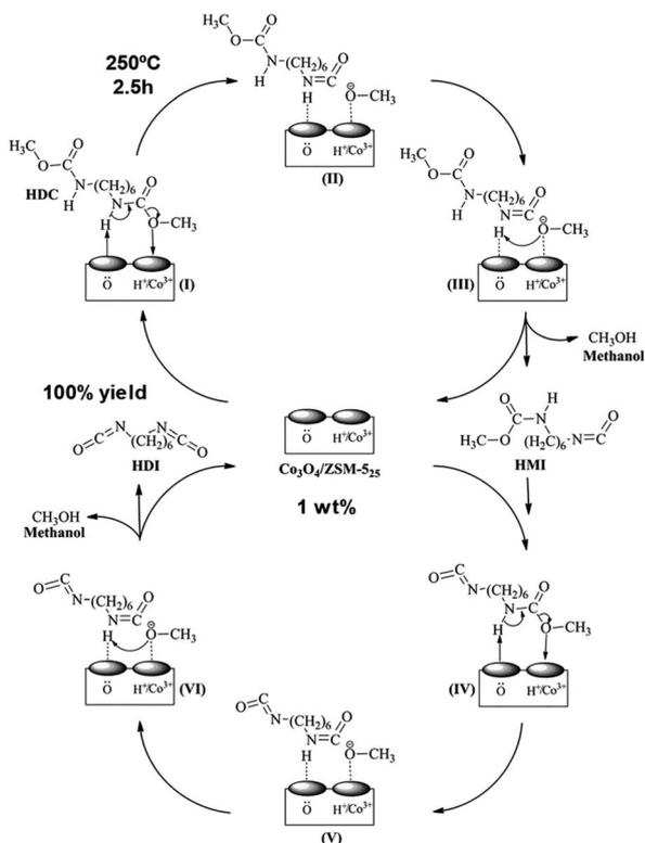
Scheme 19 A tentative mechanism for the thermal decomposition (250 °C) of HDC to HDI over  $\text{Co}_3\text{O}_4/\text{ZSM}-5$  catalyst. Reproduced with permission of ref. 90. Copyright (2017) Elsevier.
